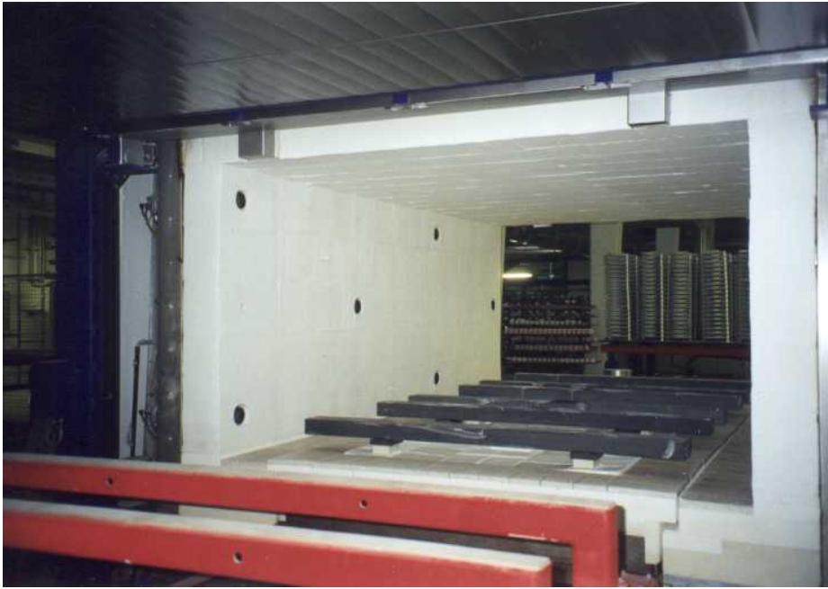
Figure 1.3: Furnace for large samples tests.
