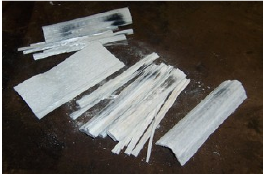
Figure 6.17: After the test the fibres of the pultrusion could be separated. No resin was left in the specimen as result of the fire exposure.
