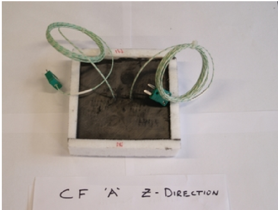
Figure 5.1: Specimen for the step change test. Insulation material prevents heat transfer through the edges to ensure one-dimensional heat flow.
