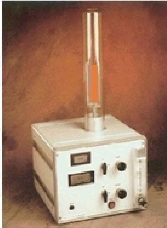
Figure 1.2: Limiting oxygen index apparatus.
