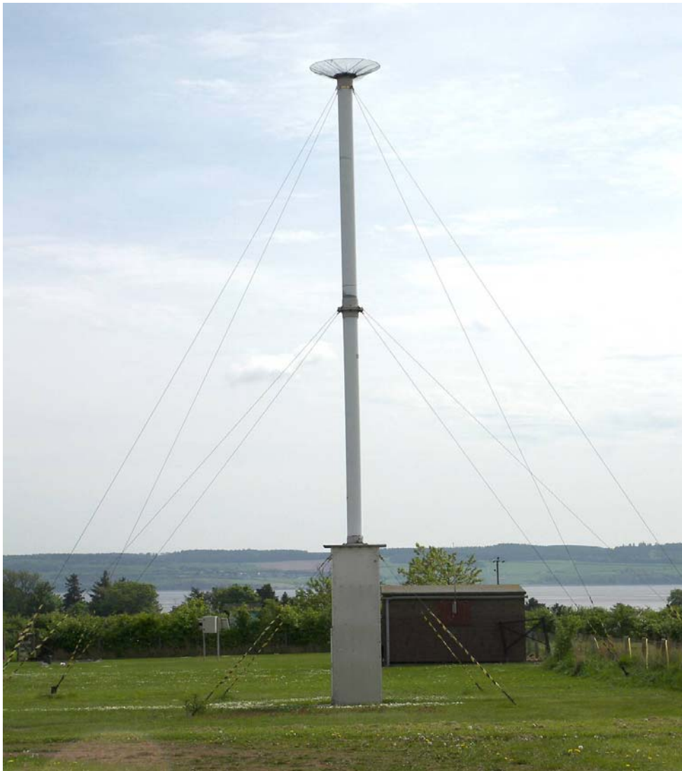
Figure 1.8. 12.2 m Rothamsted type suction trap, used to monitor aphids in the UK (SCRI).
