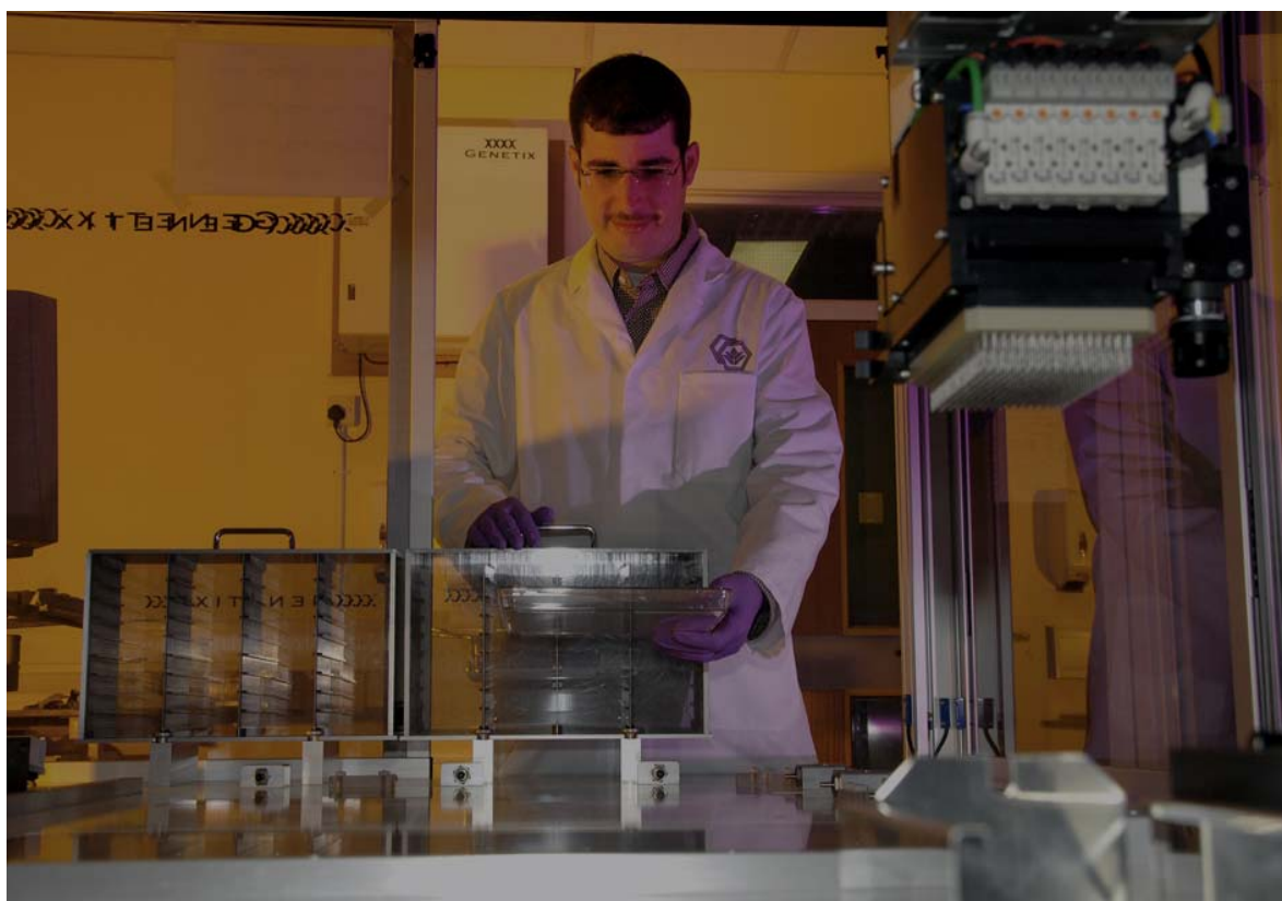
Figure 3.1. The Q-Bot robot used for the filter printing process (Picture from SCRI Annual Report, 2007).
