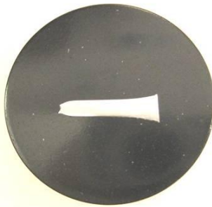
Figure 3-13. Cross-section of a fractured specimen polished for crack measurement, 1.5x
