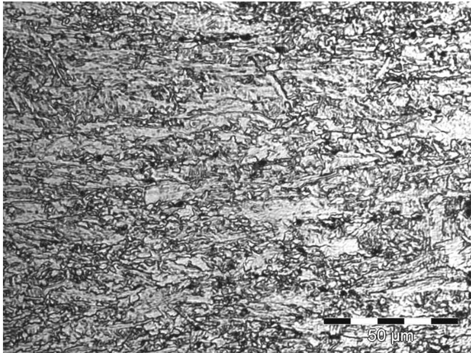
Figure 4-16. Microstructure formed at 10 mm from the centre of the grade X100 steel seam weld
