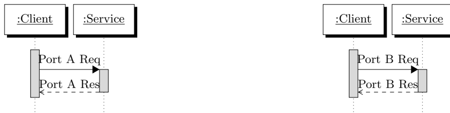
Figure I.3: Sequence diagrams representing the choices of port offered by the service component.
