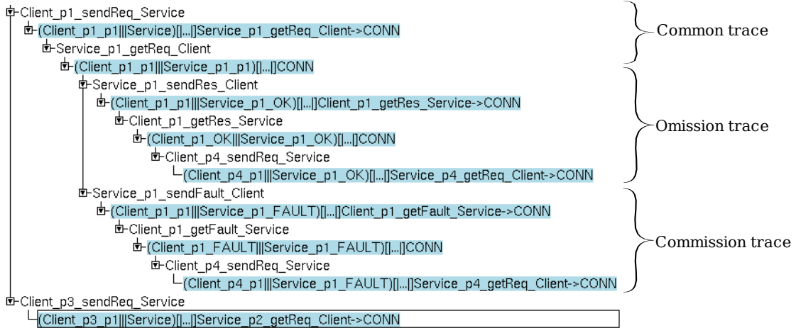
Figure 6.14: The ProBE output showing the traces possible in this system, with the trace returned by FDR for each mismatch highlighted
