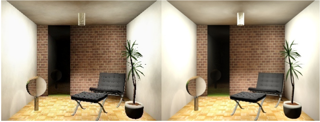
Figure 52: Left shows rendering of test model using prototype photon search CAM. This was formed by averaging 10 images, where the CAM stored approximately 3800 photons in each case. Right shows software rendering of the same model at a higher resolution. Note the difference in the renderings of the light shade, due to the averaging used with the biased photon mapping algorithm.
