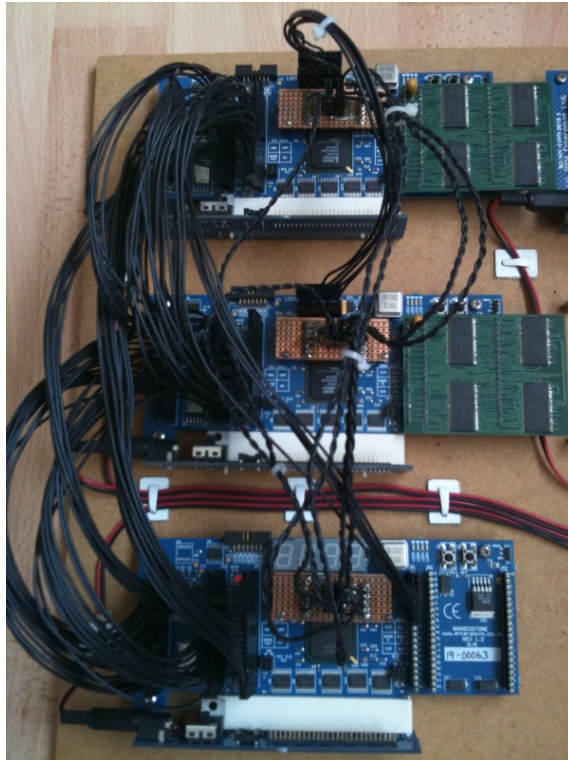
Figure 45: Photograph of prototype RTI acceleration hardware. See the attached RAM expansion modules on the development boards containing the pipeline (top and middle).
