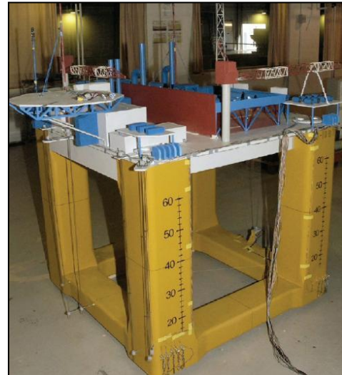
Figure 3-2 The semisubmersible scale model
