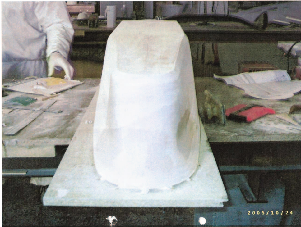
PLATE 4.4 FPSO hull prepared from fiber glass epoxy resin
