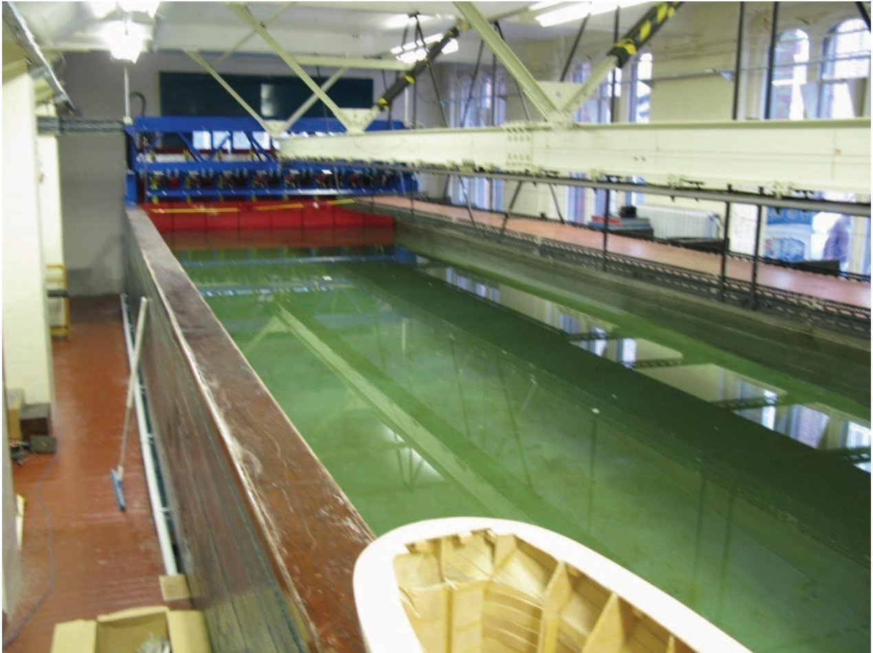
PLATE 4.1 - A section of the towing tank showing the paddles.
