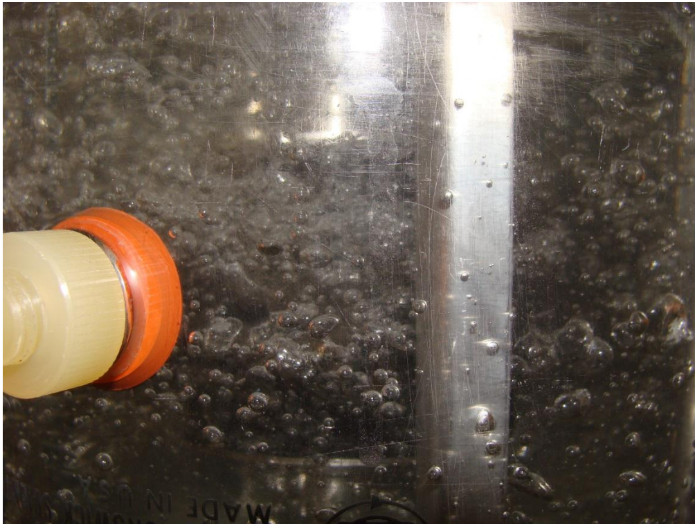
Figure 5.16a: Picture of air bubbles taken with the 6 cm Declon Mesh impeller at 200 rpm/1.0
