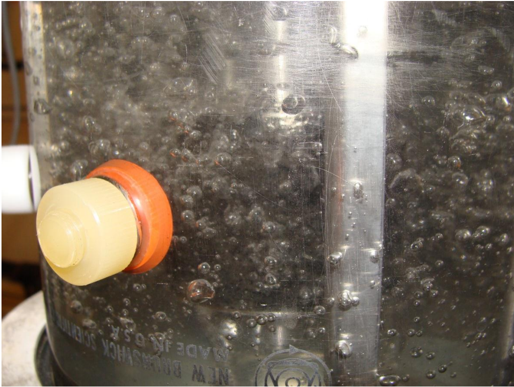
Figure 5.16b: Picture of air bubbles taken with the 6 cm Knitted Wire impeller at 200 rpm/1.0vvm
