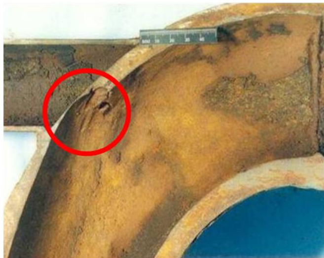
Figure 1.2: Effect of sand erosion on the pipe wall (image taken from http://ceresist.com ).
