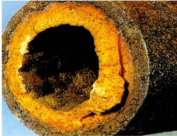
Figure 1.3: Build up of wax deposits on the walls of a pipe (image taken from http://balmsenergy.com ).
