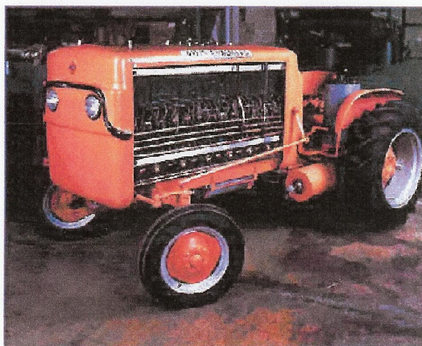
Figure 1.6. The Allis-Chalmers 1.5 kW AFC tractor in the Smithsonian museum (from Smithsonian institutions [33])
