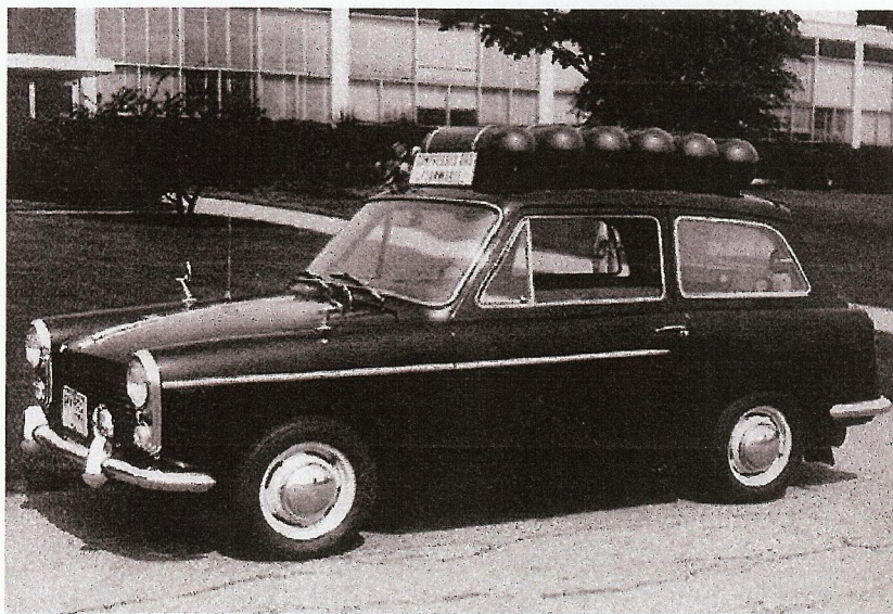
Figure 1.7. The Austin A-40 hybrid car of K. V. Kordesch. Six hydrogen bottles were mounted on the roof, the 6 kW H_2 -Air fuel cell system was in the rear, lead-acid batteries were under the bonnet [21].
