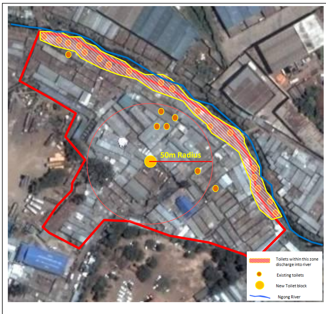
Figure 7-2 New Toilet Facilities in Fuata Nyayo Village, Mukuru
