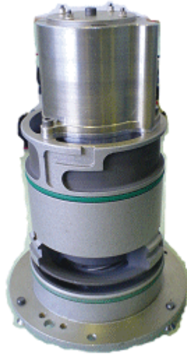
Figure 87 - A320 Induction motor pump
