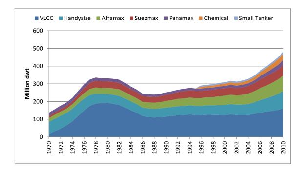
*Figure 1.6 Tanker fleet capacity (16% growth a year for chemical and small tankers)*
