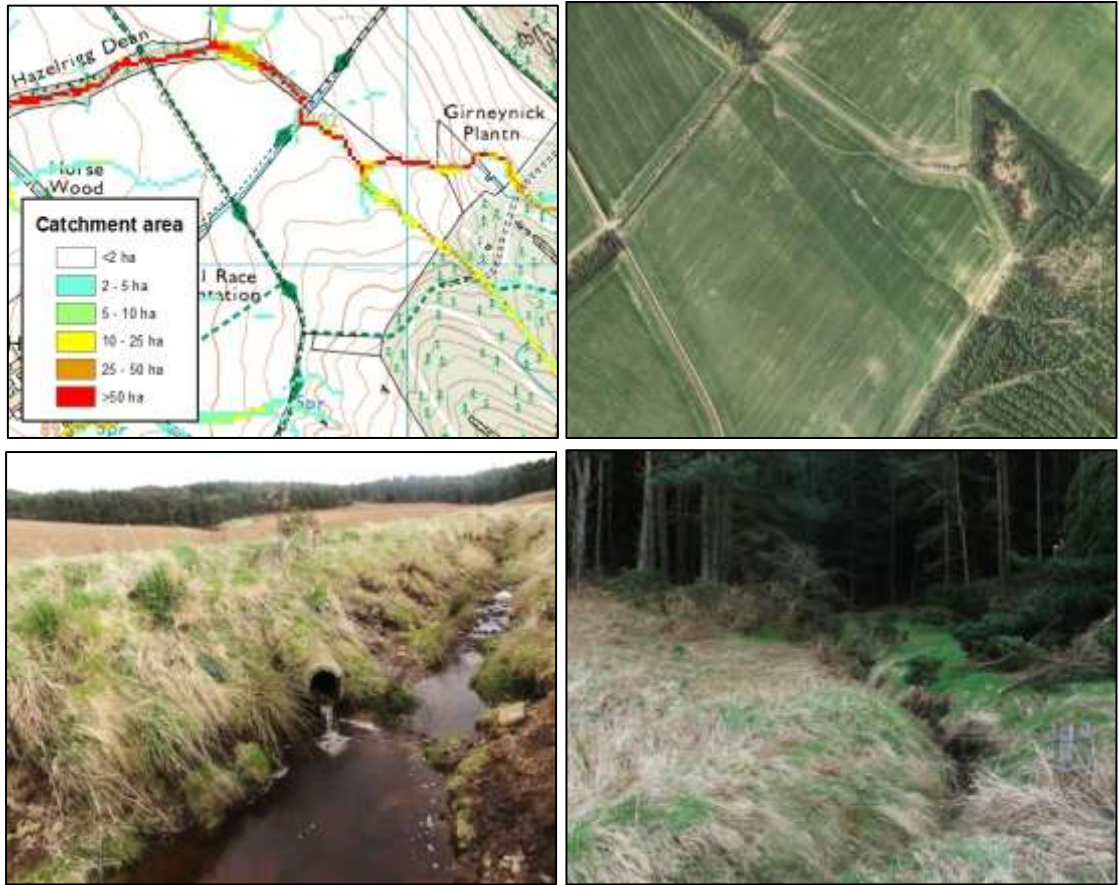
Plate 6.4: Clockwise from top left: Contributing area; erosion 2002; stream exiting woodland to east of field; permanent gully feature 2011 (piped stream outlet from northern flow path).
