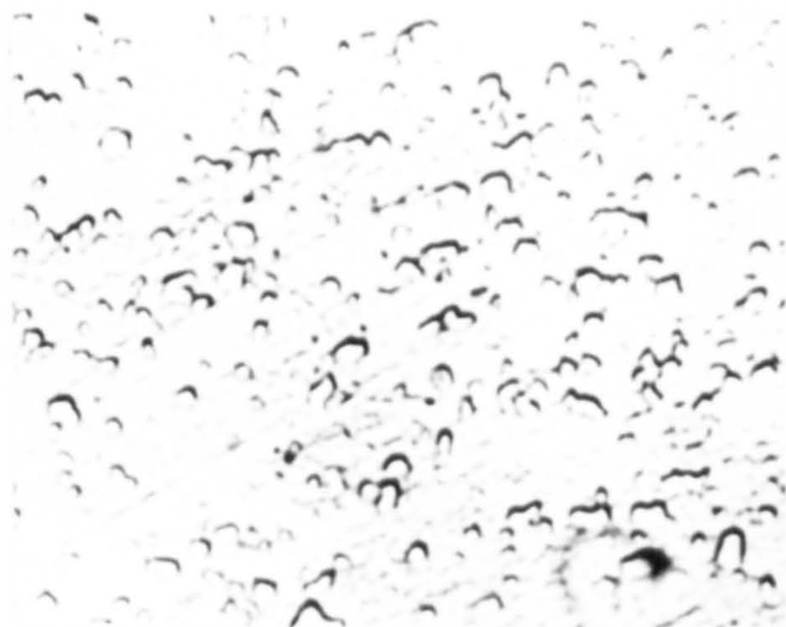
(a) Fe-9.3 wt.% W annealed 3 h. at 880 °C \alpha + \text{Fe}_2\text{W}
