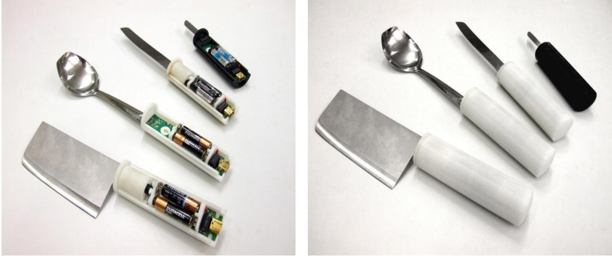
Figure 3.2: Utensils instrumented using a modified Wii Remote.
