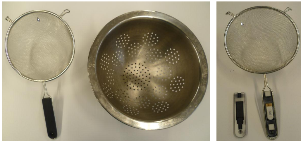
Figure 6.4: Wax embedded sieve and colander (left); opened sieve (right).
