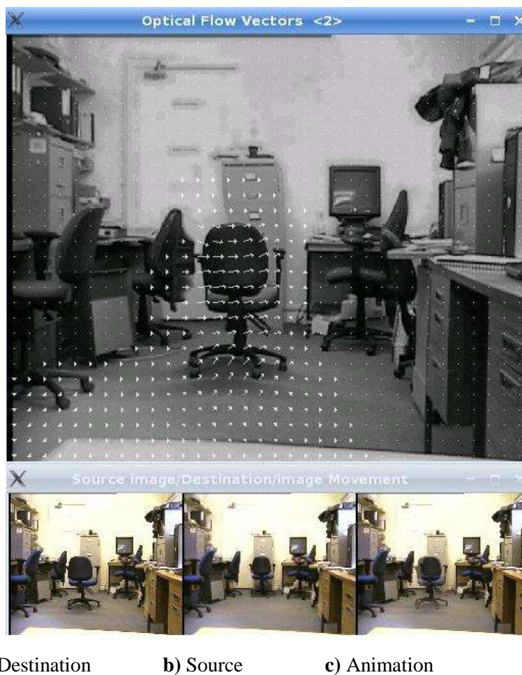
Figure 3.1: Illustration of flow vectors and motion animation, (a) destination image, (b) source image, (c) movement animation
