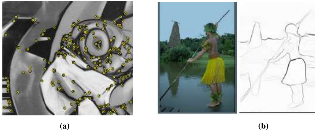
Fig. 4.1: Illustration of local features in gray-value and coloured images (a) Interest points with corner detection [Tuytelaars and Mikolajczyk 2008], (b) Contour detection [Maire, 2009]
