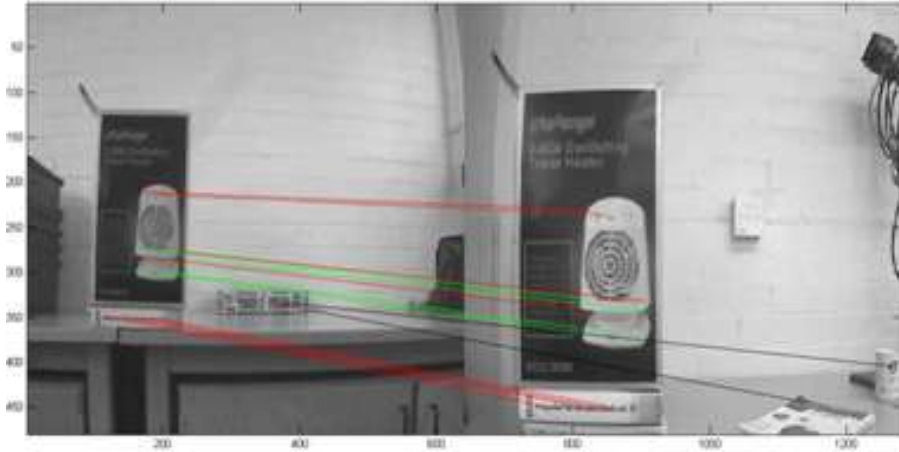
Figure 5.3: Matching example, including different clusters (1 th cluster (black), 2 th cluster (green), 3 th cluster (red))
