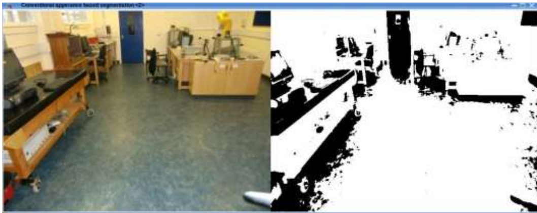
Figure 3.10: Appearance-based obstacle detection method
