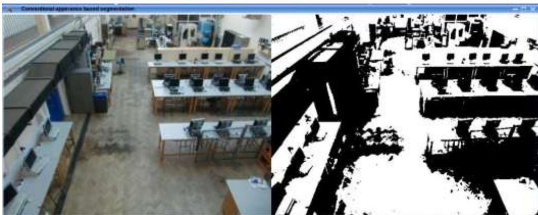
Figure 3.11: Effects of lighting conditions and unexpected stains on the floor
