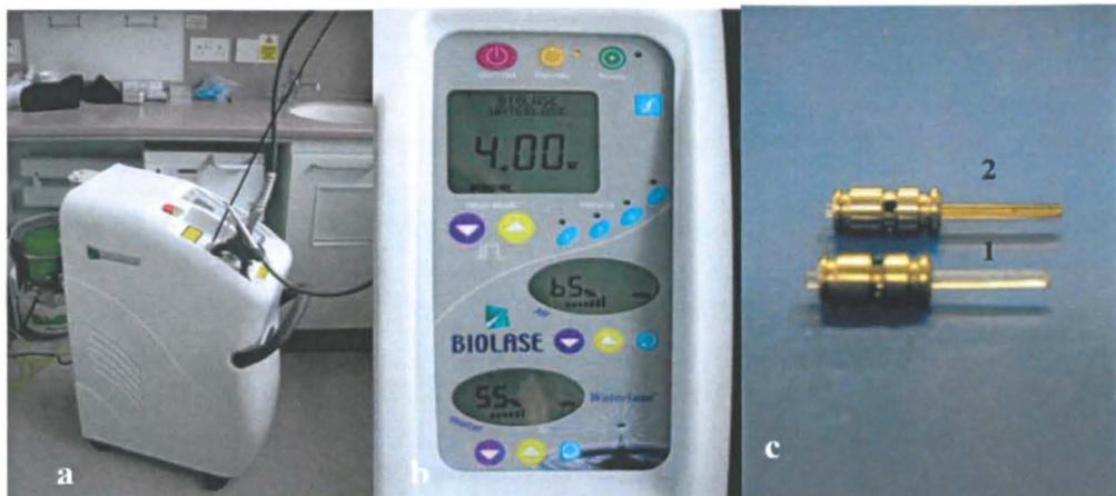
Figure 3.1 (a) The Er,Cr:YSGG laser unit (b) Control Panel showing power settings, as well as percent of air and water during the cutting process (c) The sapphire tip (1) and zirconia tip (2).
