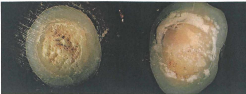
Figure 4.12 Light microscopy showing two types of failure a) Adhesive failure and b) Mixed failure
