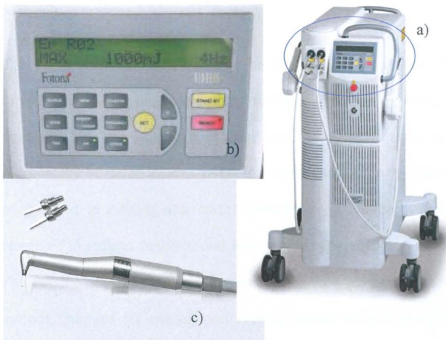
Figure 1.7. a) Er:YAG laser unit b) The laser tip on the handpiece with water spray cooling system c) the control panel showed the energy and repetition rate (retrieved from the website [www.ondanet.it/forb/azienda\\_04.html](http://www.ondanet.it/forb/azienda_04.html) May 2007)
