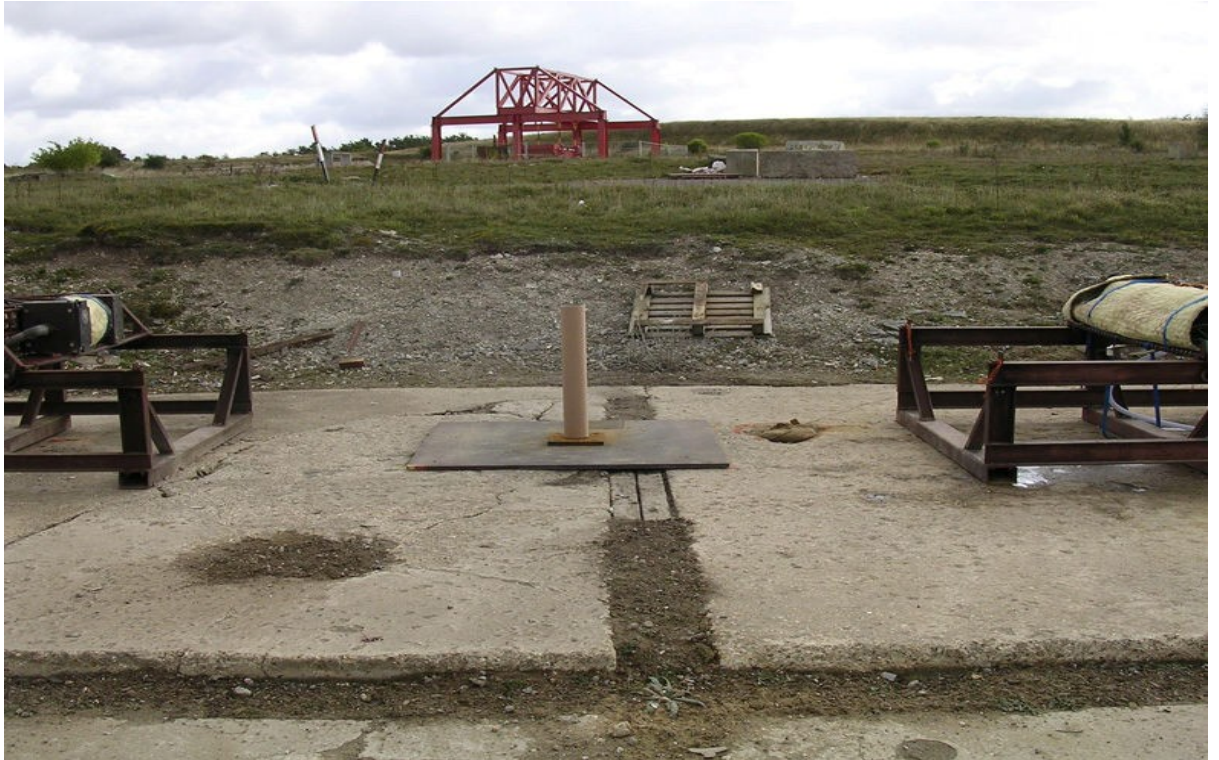
Figure 21: Photograph of blast arena. Charge was fastened to central cardboard tube and the animal positioned on trolley to the right wrapped in Kevlar blanket.
