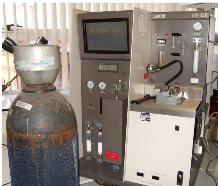
Figure 37: Leco FP428 nitrogen analyser
