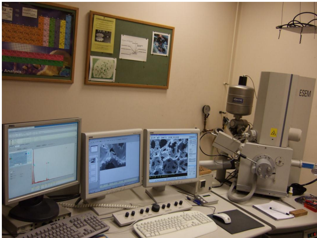
Figure 15: Cambridge s240 scanning electron microscope
