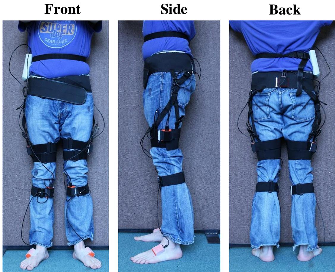
*Figure 6.1 Sensor attachment positions for Xsens MTx sensor using custom-made Velcro straps.*
