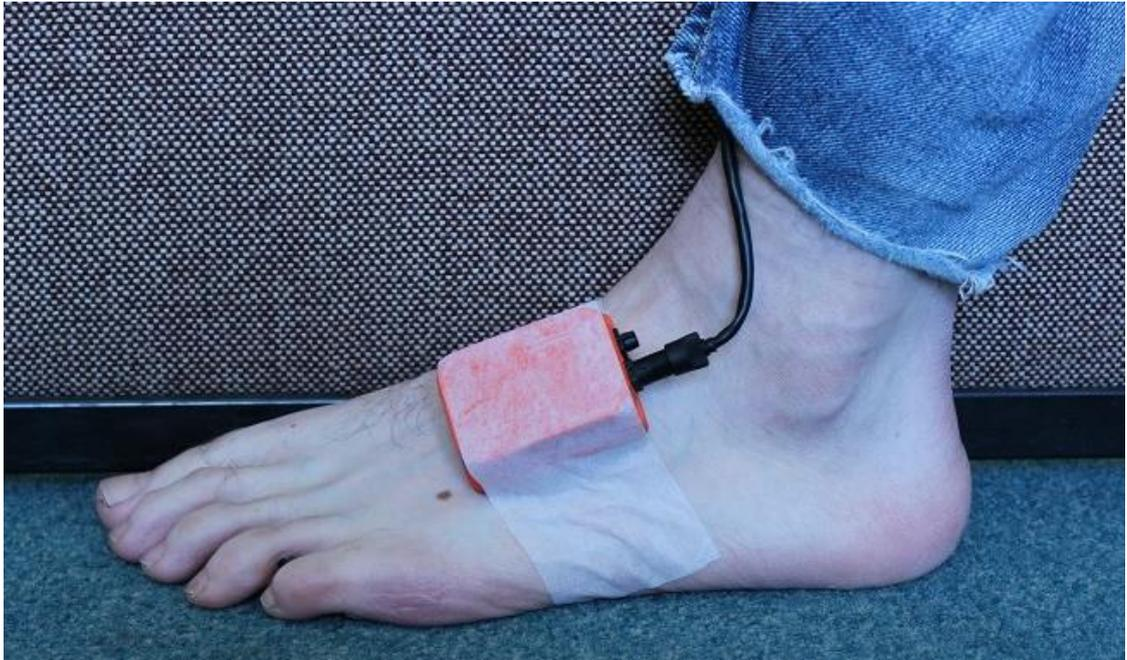
*Figure 6.2 Attachment of MTx sensor to dorsal surface of foot using double-sided tape and surgical tape.*
