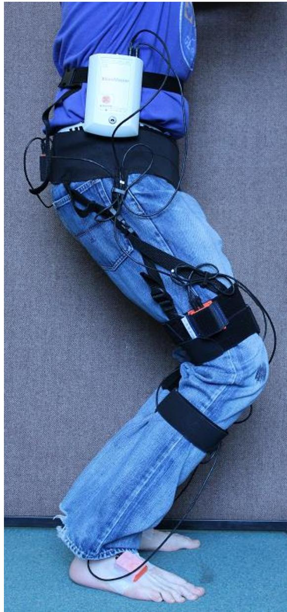
*Figure 6.6 Squat calibration movement used to calibrate the thigh and shank sensors.*
