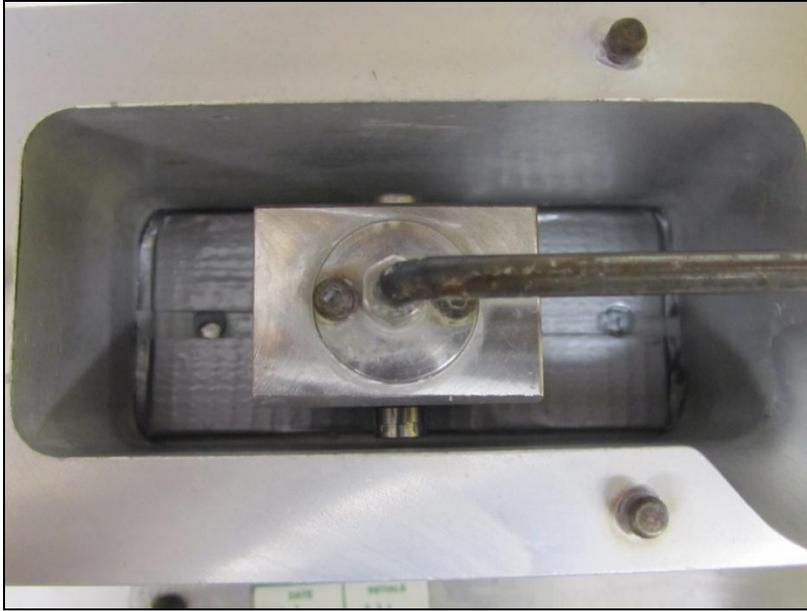
Figure 28. Composite specimen in a water bath of toothbrush simulator.
