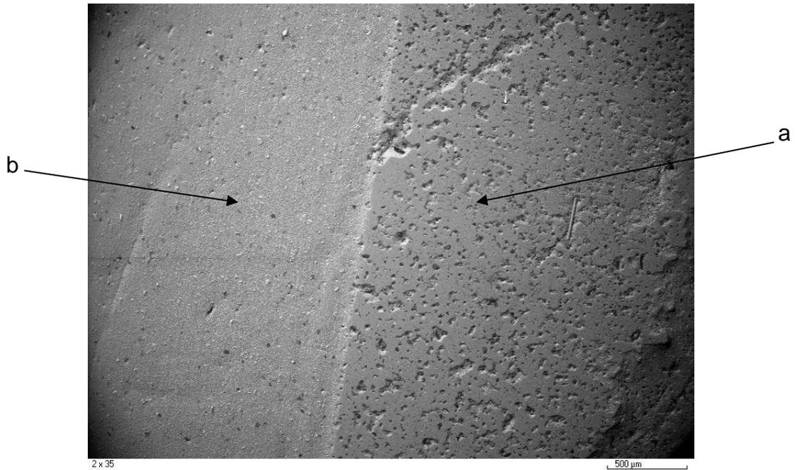
**Figure 36. Build It after 24 hours water storage and 50,000 TB cycles (SEM image x35): (a) is the unbrushed surface, while (b) is the brushed surface.**
