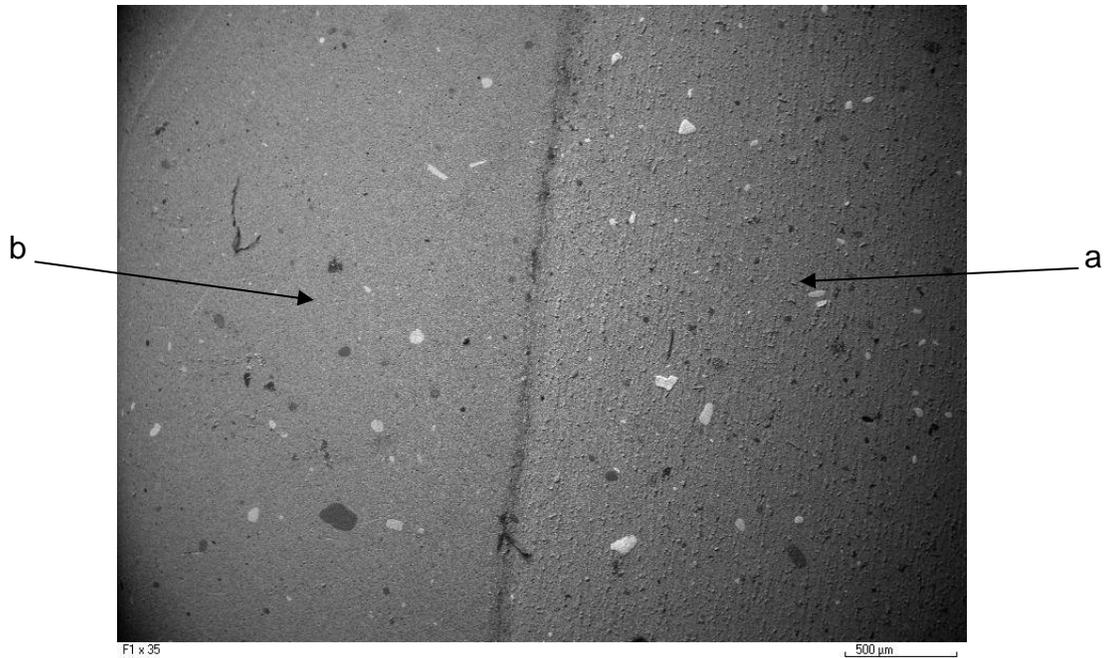
**Figure 38. Build It after 1 year water storage and 50,000 TB cycles (SEM image x 35): (a) is the unbrushed surface and (b) is the brushed surface.**
