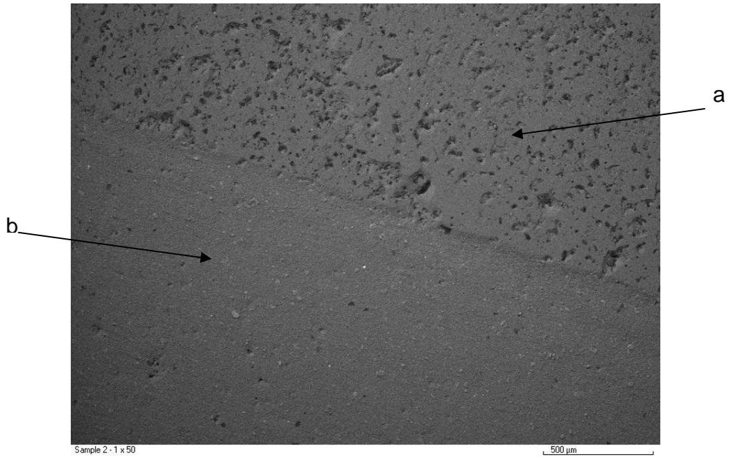
**Figure 40. Z250 after 24 hours water storage and 50,000 TB cycles (SEM image x 35): (a) is the unbrushed surface and (b) is the brushed surface.**
