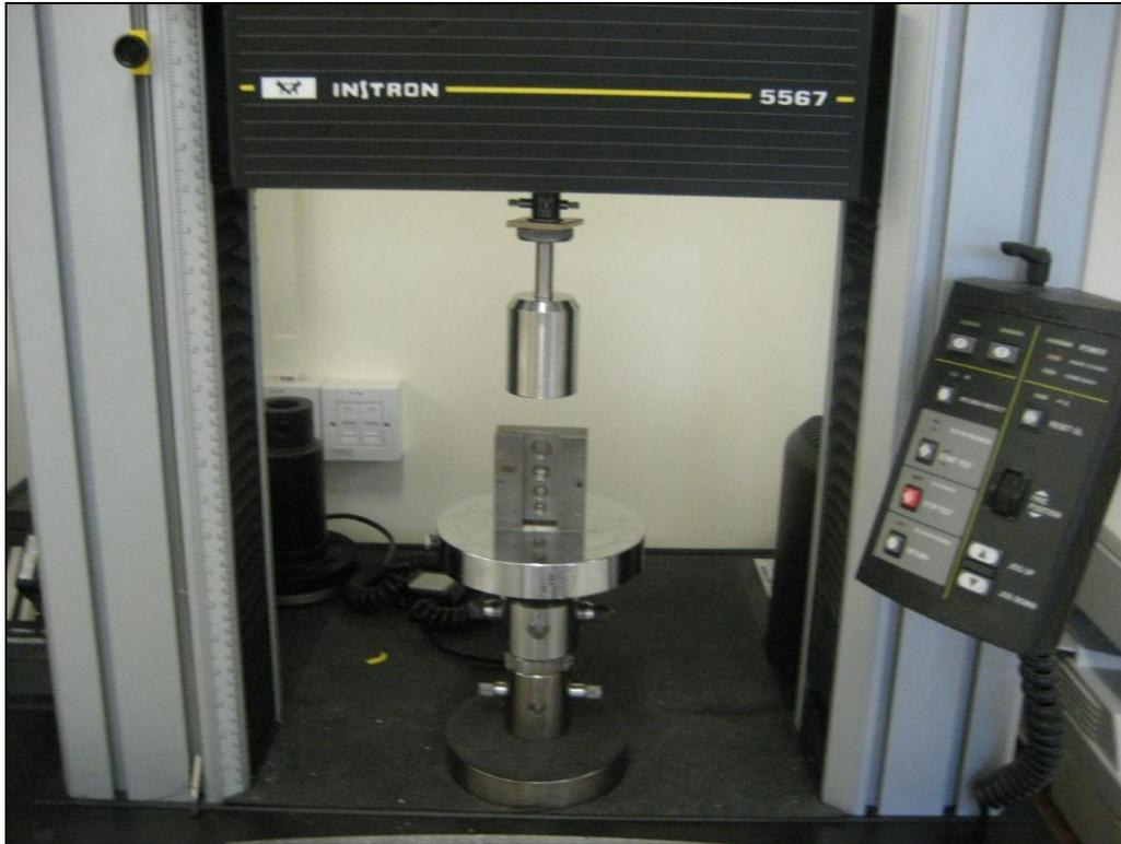
Figure 57. Instron 5567 used for shear bond strength (SBS) testing.
