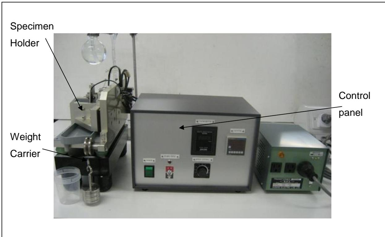
Figure 4. Rolling ball machine basic components.
