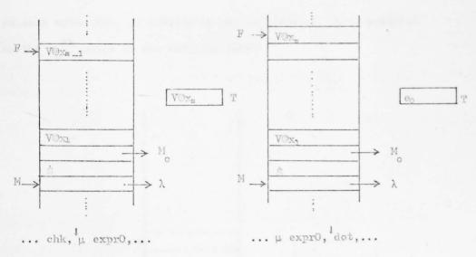
The value of the function body, expr0 is left in register T after evaluation. Note that this may have involved arbitrarily many function calls, nesting the marks, but that the integrity of the information stored here will have been retained (if vectors are used incorrectly however, it is possible to interfere with this information since the subscript is not checked for range).
