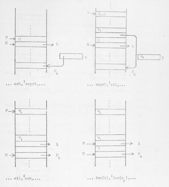
At this stage, neither the value of T nor the value of P is correct in the sense of their specially defined roles. Indeed T is not in use and F is being used to run up the actual parameter list. After executing for  $(x_j)$ , each of the elements  $VPx_1$ , ..., VPx has been reset to contain  $e_1$ , ...,  $e_j$  respectively, while the state of the stack is as follows:
