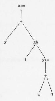
and hence the values of x and y are incremented and exchanged.
