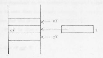
After X = nY the register X points to the next element to that pointed to by Y. For example, F = nF moves the stack top pointer up.
