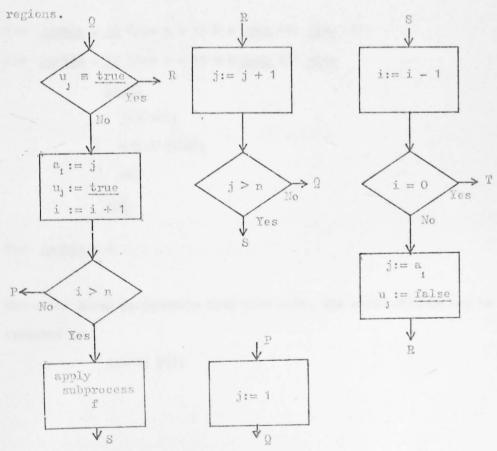
Because of this tree-like structure, and because the exit from each region identifies a successor region, we can encode each region as a parameterless function in an obvious way.
