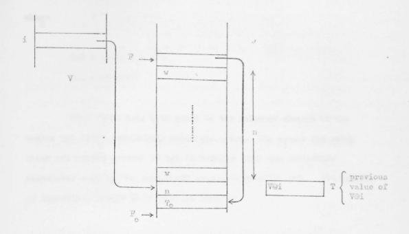
To and Fo are the initial values of T and F, n is the value of expr1 and w the value of expr3 (or undefined in case the vector is not to be initialised). Note how a link is placed on the stack after the vector in order to "down date" correctly. This is in order not to have to rely on the value of VDi which might be changed by assignment.
