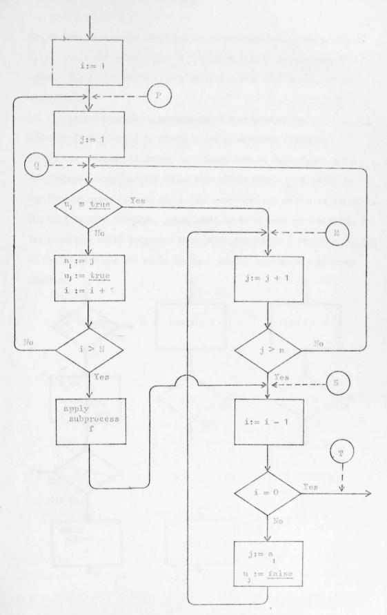
The diagram represents an algorithm to generate permutations of 1,...,n and submit them to the subprocess f in lexicographic order. The algorithm is described fully along with Example 11 in Appendix 3.
