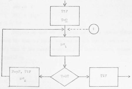
We postulate that there exist functions  $\alpha$  and  $\beta$  with the property that, if we enter the diagram at 1 with  $\xi = [t,f,v]$  then we exit (if at all) with the environment
