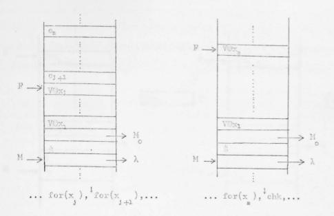
Note how m actual parameters are obtained by ignoring  $e_{n+1}$ , ...,  $e_n$  if  $n \ge m$  or by taking arbitrary values from the stack if  $n \le m$ .
