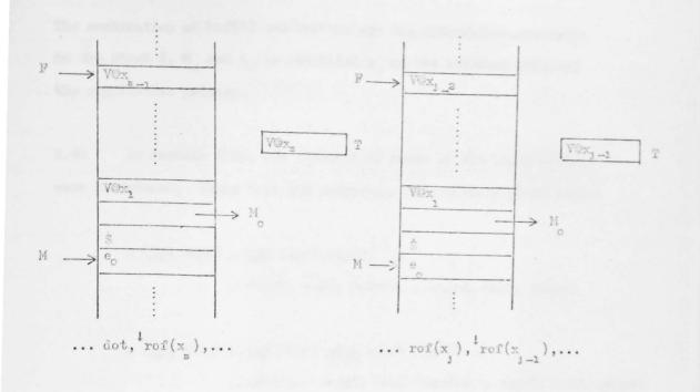
As each value  $V \odot x_j$  is removed by rof  $(x_j)$  from T, it is restored to the  $x_j$  th entry in the variable table
