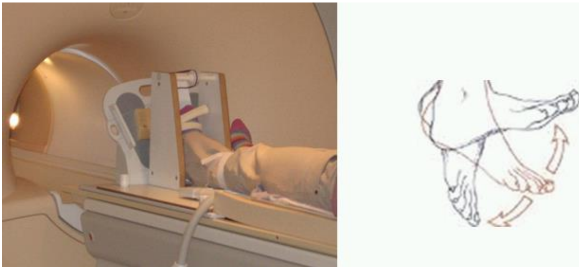
Figure 20 illustrates the apparatus used to permit exercise (plantar flexion) within the MR scanner (left) and the 0°-30° of plantar flexion involved (right)
