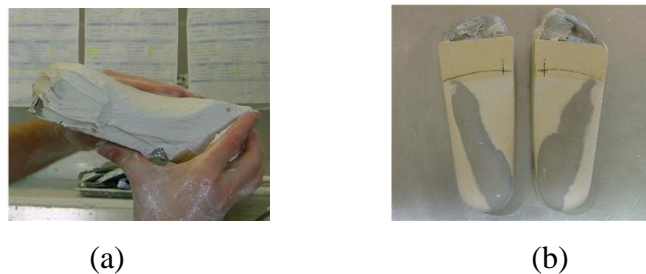
Figure 2:31 Manual corrections process in positive mould (a) and (b) corrected positive mould with arch fill design feature (footcraft.com.au, 2010)
