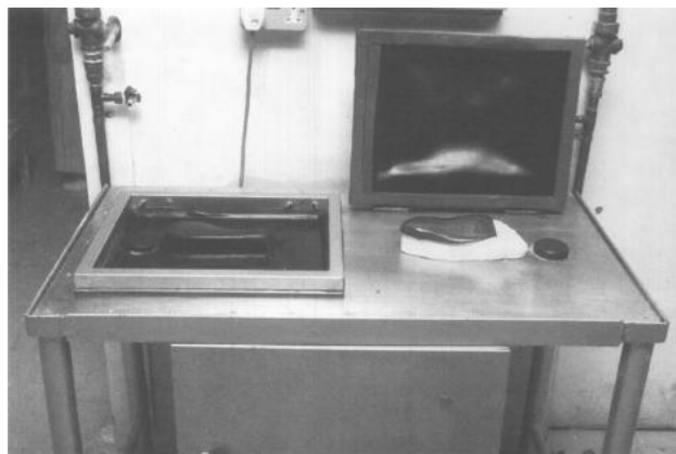
Figure 2:34 Vacuum press and moulded orthoses shell (Pratt, 1995)
