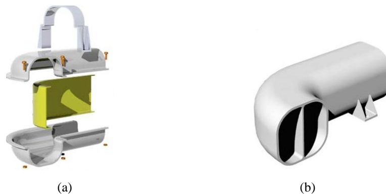
Figure 2:9 Aircraft duct (a) original design with 16 parts (b) consolidated design (Gibson et al, 2010)
