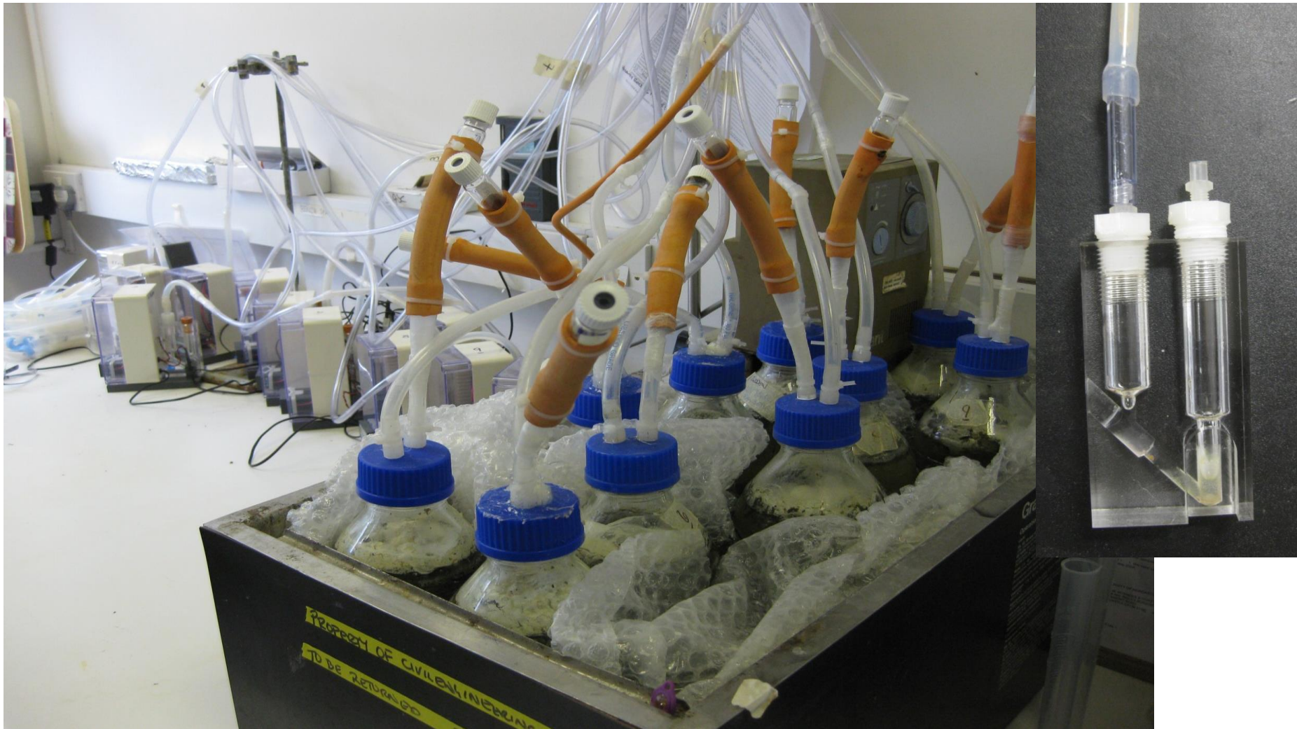
Plate 8.1 Anaerobic digester experimental set-up, showing water bath, digester bottles and bubble counter with detail of Perspex bubble maker and fittings in insert picture
