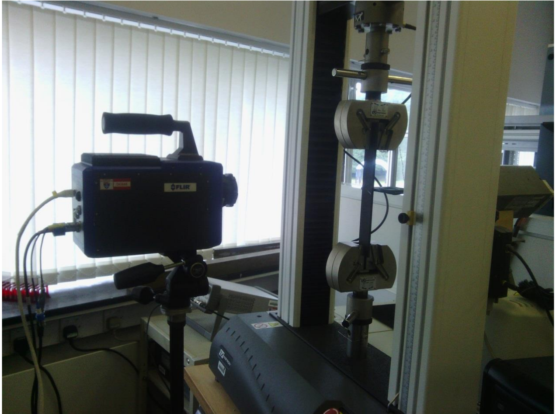
Figure 5.12 Instron model 3369 universal test machine and Flir thermal camera.
