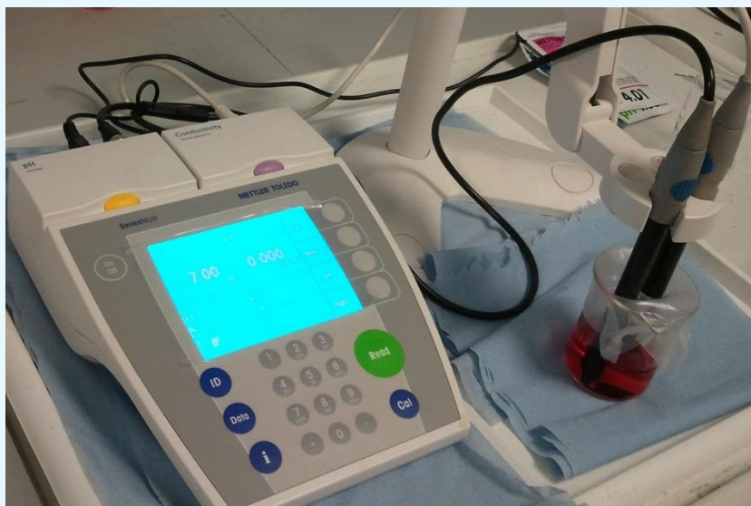
Figure 4.15 Dual pH and conductivity meter used to measure physicochemical properties of the electrolytes
