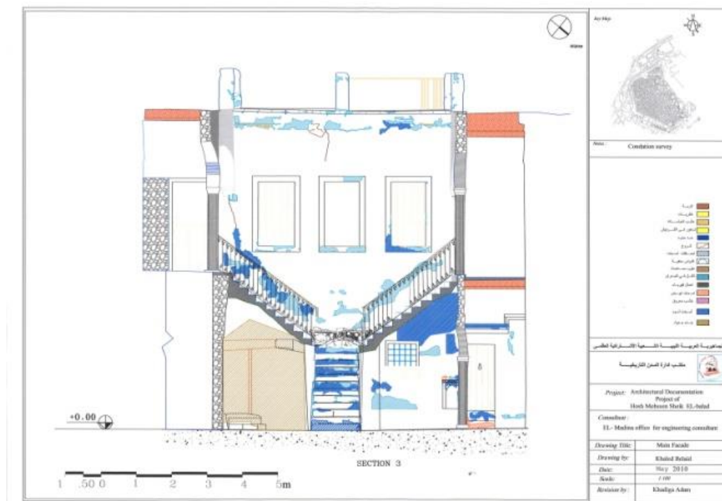
Figure 7.8: Conditional survey drawing: Hosh Mohssen in the old city of Tripoli (the MHCBC, 2010)
