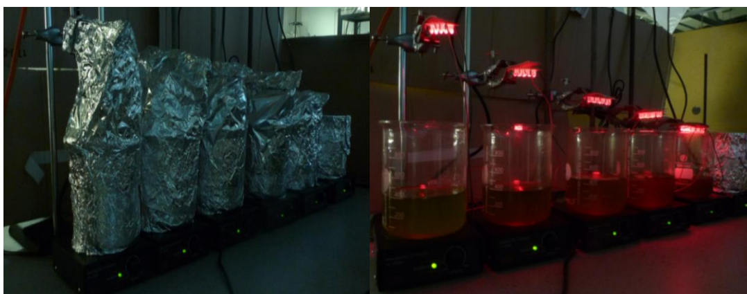
Figure 3.1 Experimental set-up (left: bioreactors covered with aluminium foil; and right: without aluminium foil cover)
