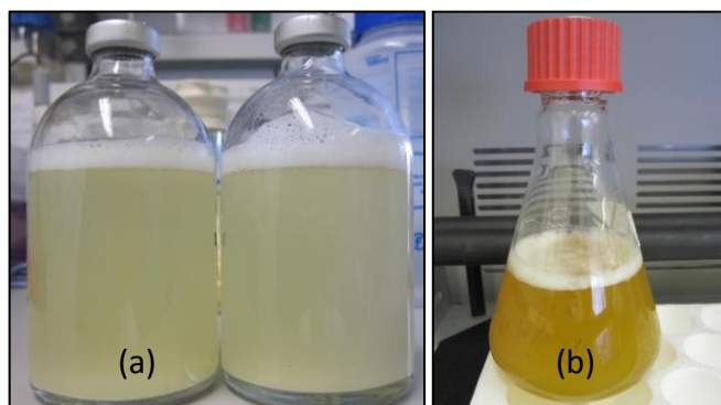
Figure 3.1 Grown inoculum developed in (a) 100 mL serum bottles and (b) 250 mL screw capped conical flask
