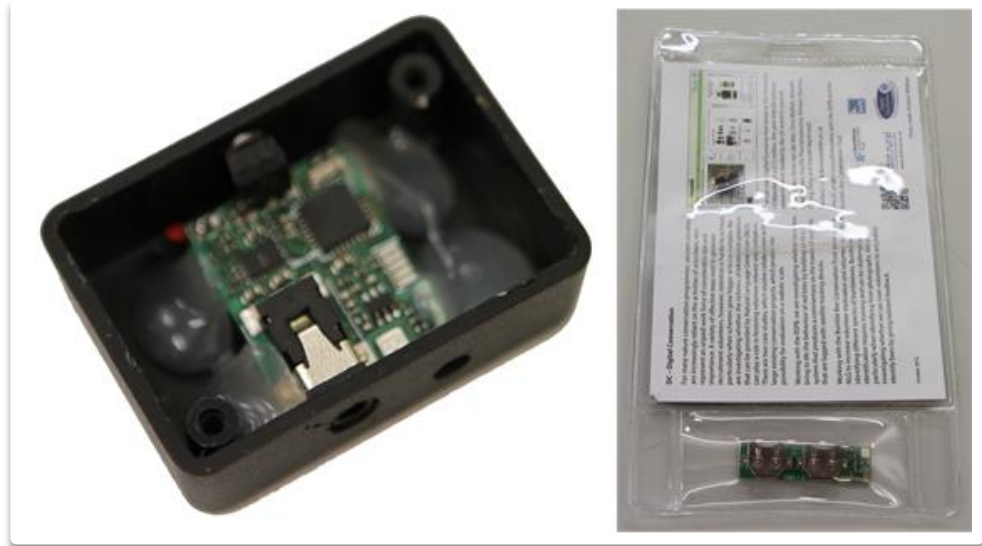
Figure 36 RedTag Emitter in a Badge and Receiver on a Camera
