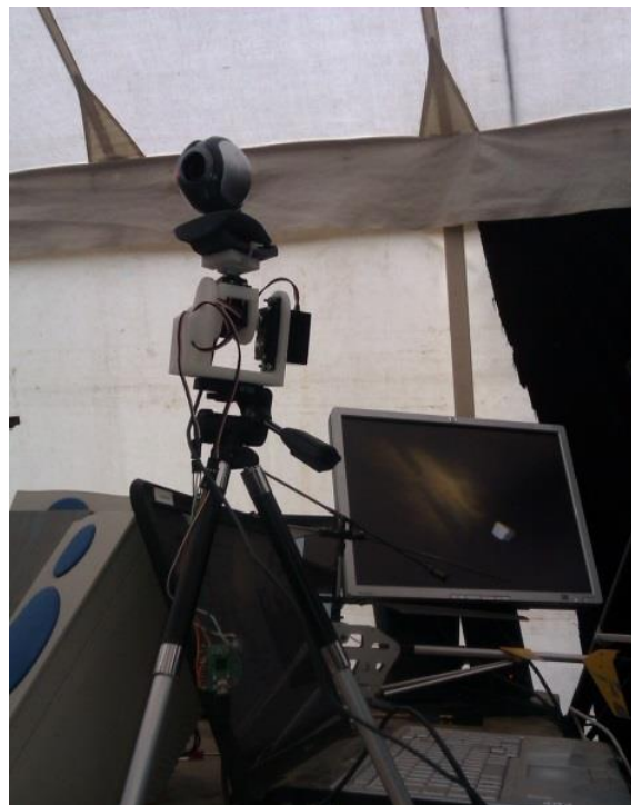
Figure 63: miniature motorized camera mount to enable live cameras to be used in Cinejack
