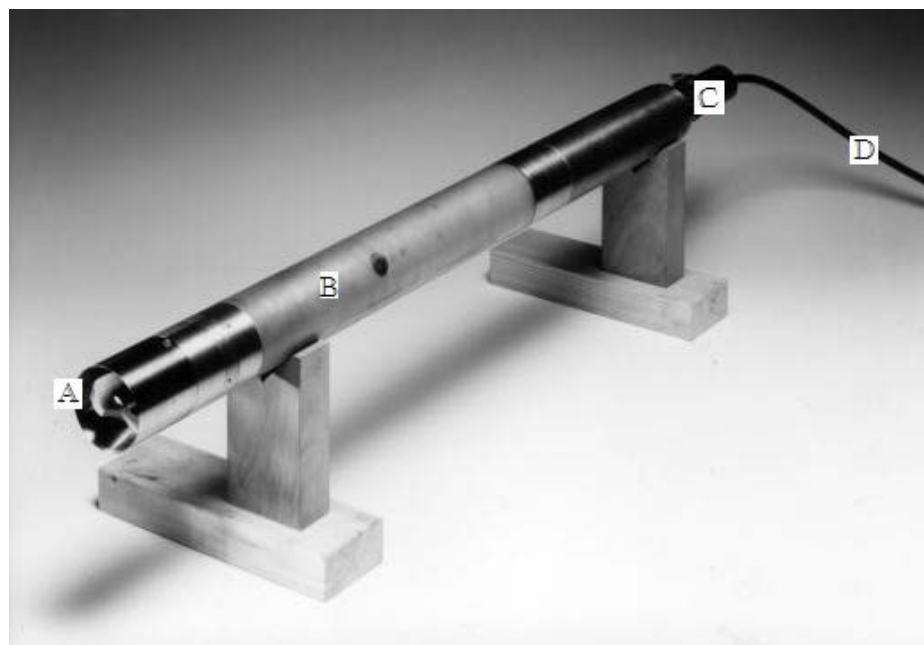
Figure 4.2: The SBPM, showing the cutting shoe (A), the inflatable membrane (B), crossover (C) and umbilical (D). Source: Adapted courtesy of CAM-INSITU .
