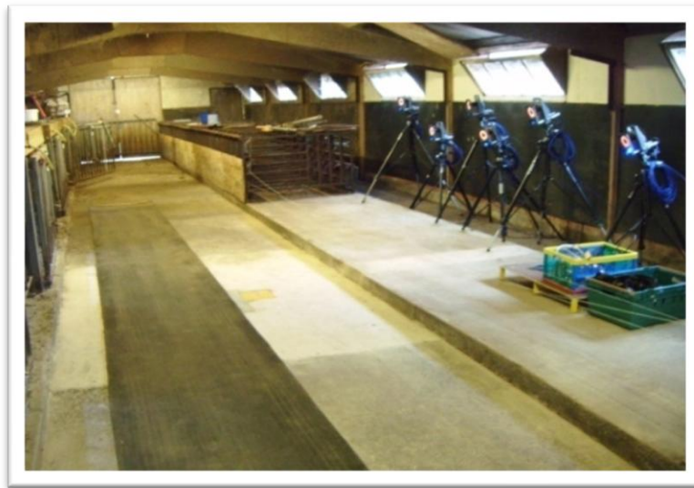
Figure 8.7: Vicon T20 camera set up for pig motion capture at the Newcastle University pig unit.
