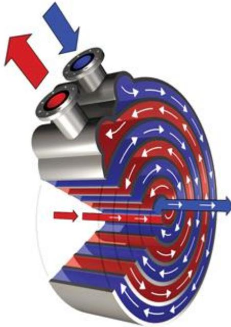
**Figure 3.9. Spiral plate heat exchanger (Alfa Laval, 2013)**
