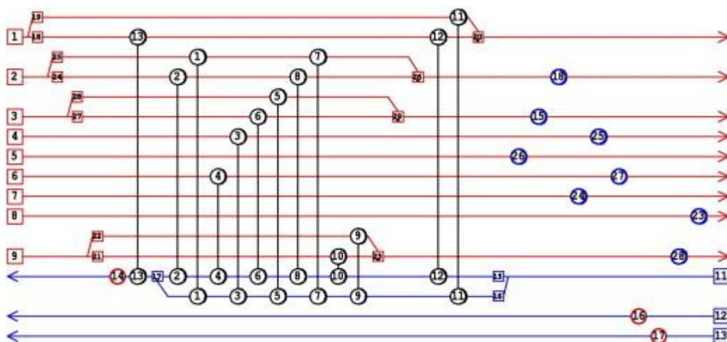
Figure 2.2. Example of a heat exchanger network map (Smith *et al*, 2010)
