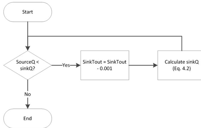
**Figure 4.15. Routine to calculate heating duties and reduce duty incrementally when no phase change occurs**
