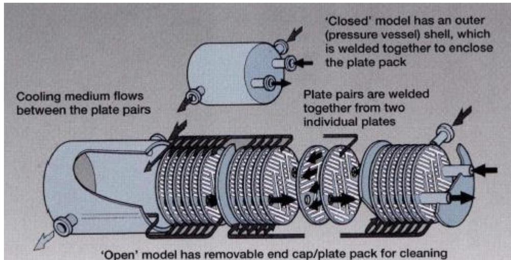
**Figure 3.8. Plate and shell heat exchanger (Best Practice Programme, 2000)**
