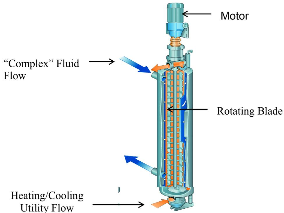
**Figure 3.10. Scraped surface heat exchanger (adapted from RheoHeat, 2013)**
