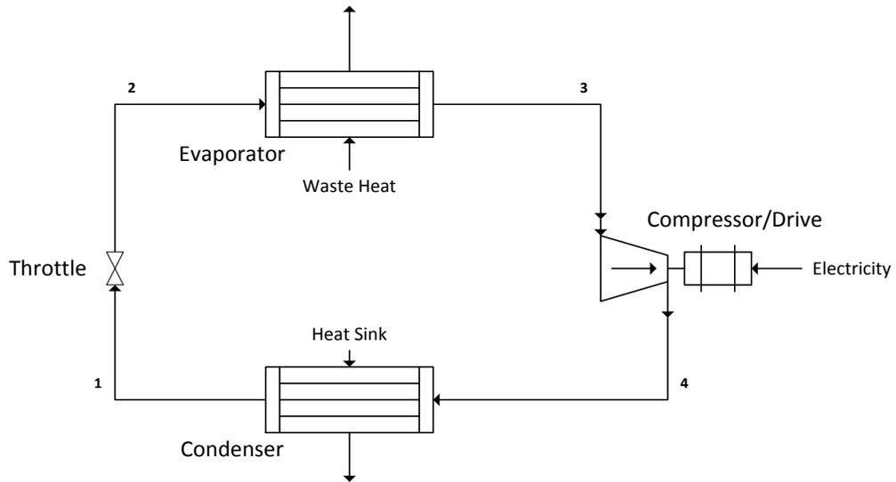
**Figure 3.14. Standard vapour compression heat pump**
