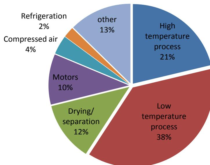
**Figure 1.5. Energy consumption by process (adapted from Reay and Morrell, 2007)**
