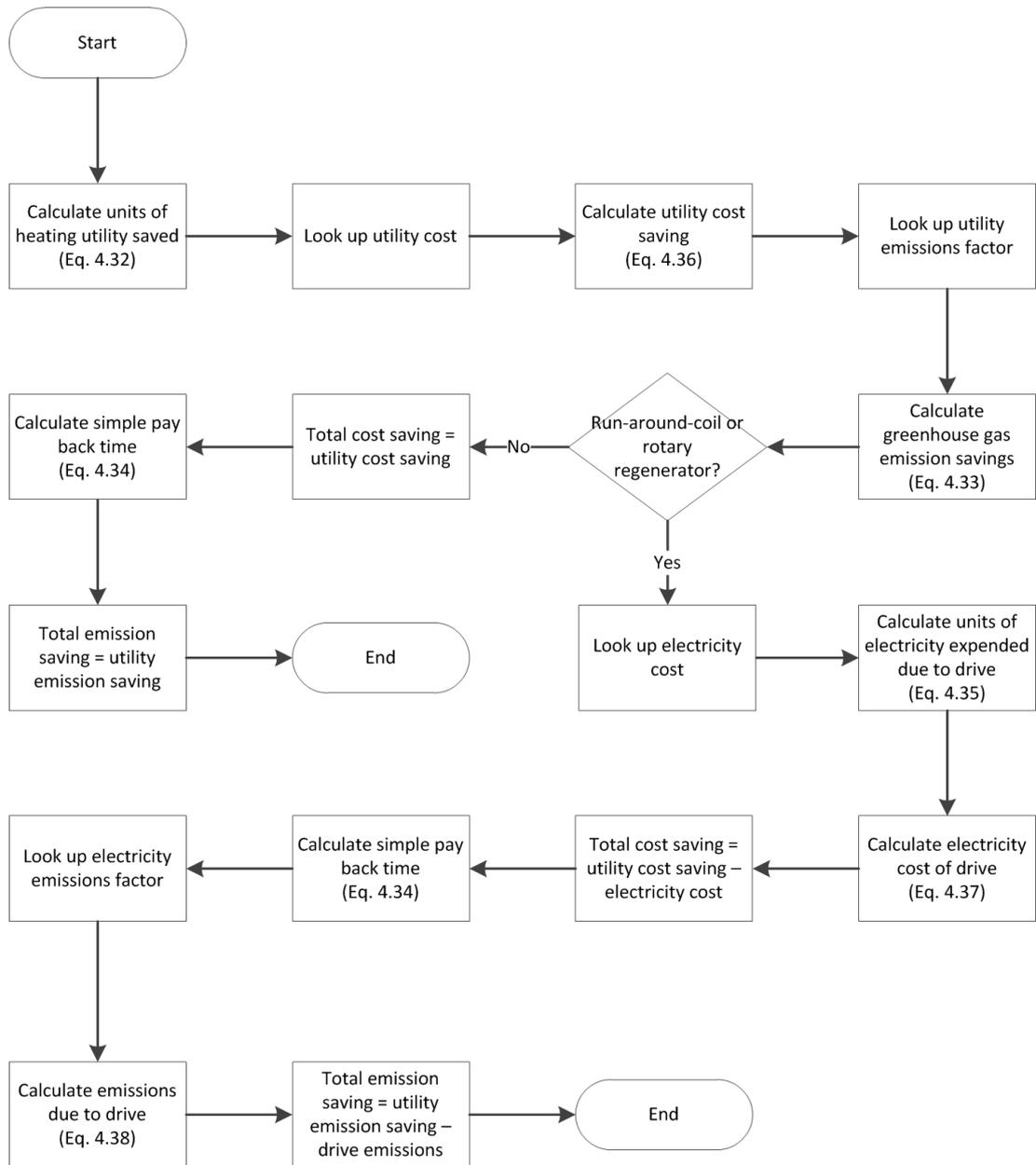
**Figure 4.20. Routine for calculating utility savings and associated benefits in heat exchanger design**
