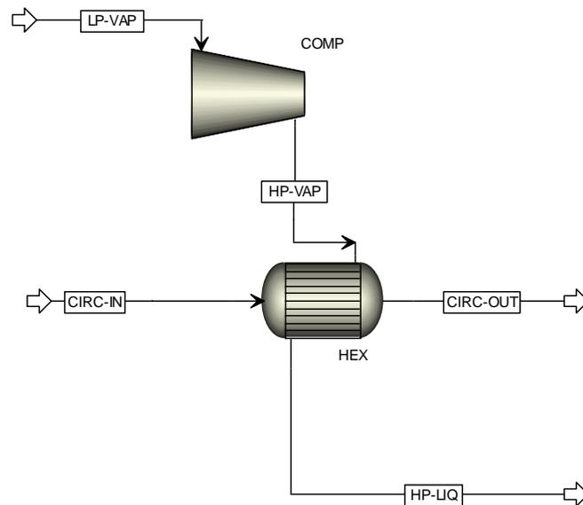
**Figure 6.6. Simplified MVR model in Aspen Plus**
