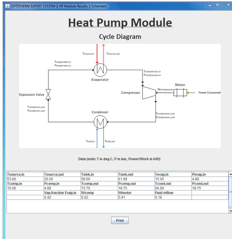
Figure A5.11. Heat pump cycle diagram for case study
