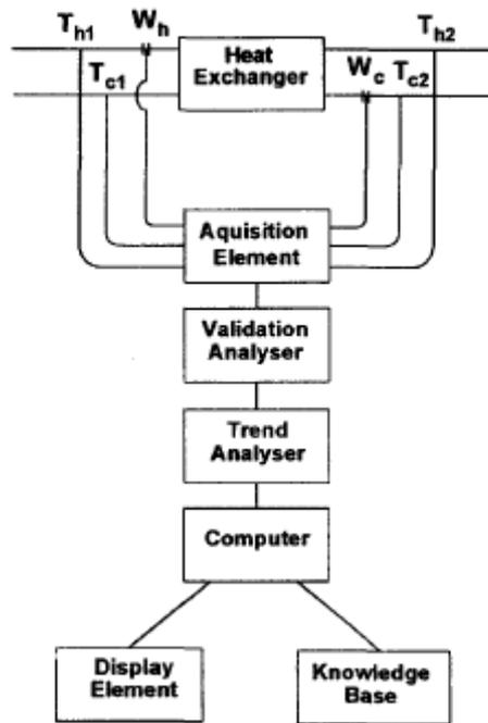
**Figure 2.7. Flow diagram of expert system by Afgan and Carvalho (1995)**
