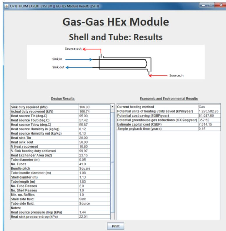
Figure A5.17. Shell and tube heat exchanger design results for case study
