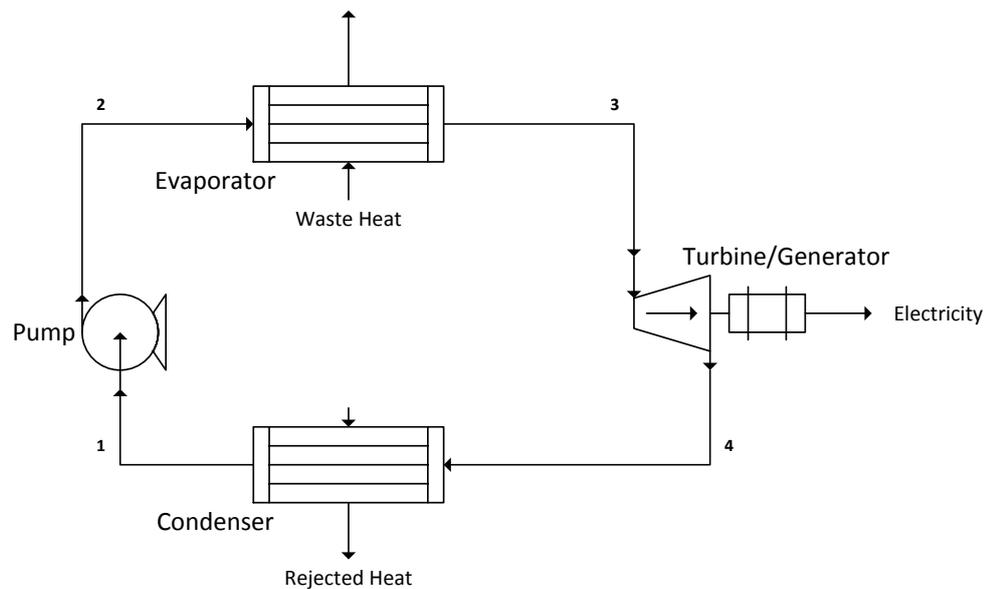
**Figure 4.27. Standard ORC configuration**
