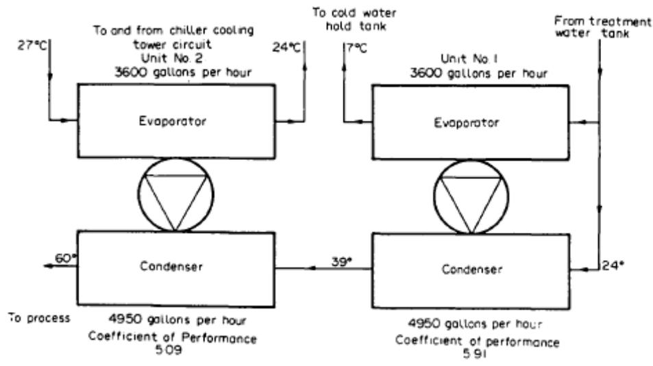
**Figure 3.15. VC heat pump providing simultaneous heating and cooling (Smith, 1983)**
