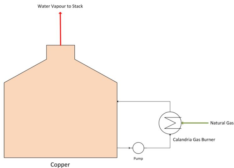
**Figure 6.5. "Wort boiling" process from case study 4**
