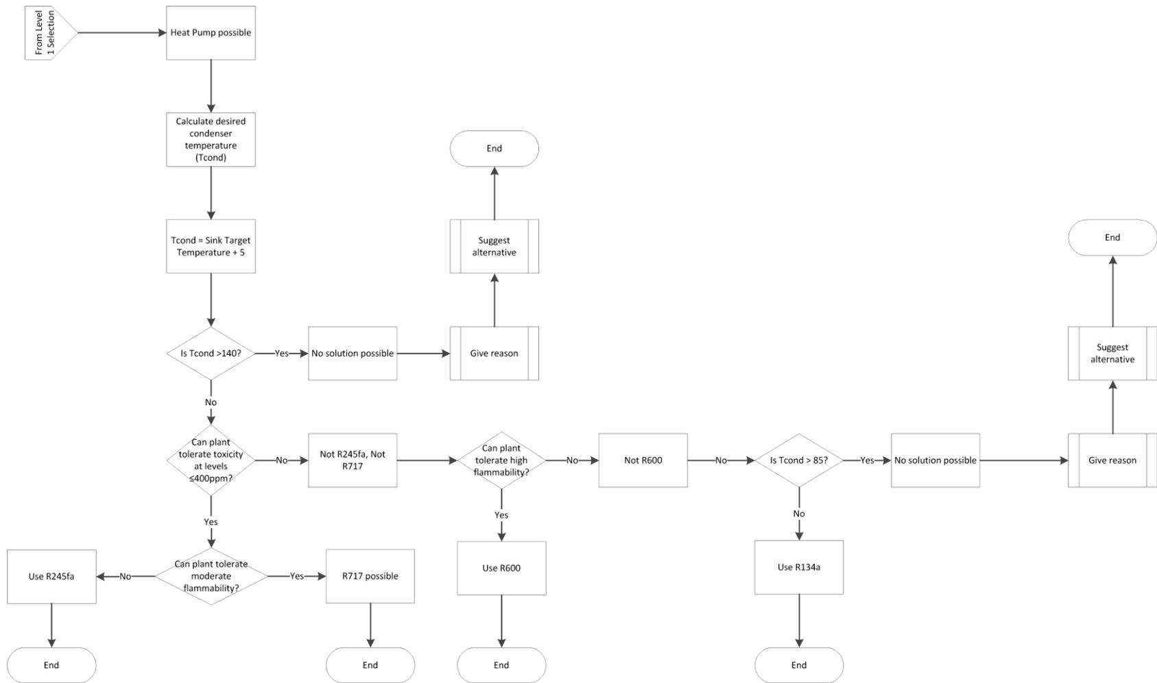
Figure 4.12. Heat pump working fluid selection knowledge-base
