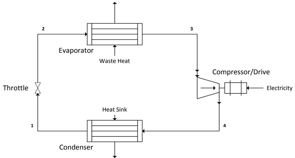
**Figure 4.21. Standard vapour compression heat pump configuration**
