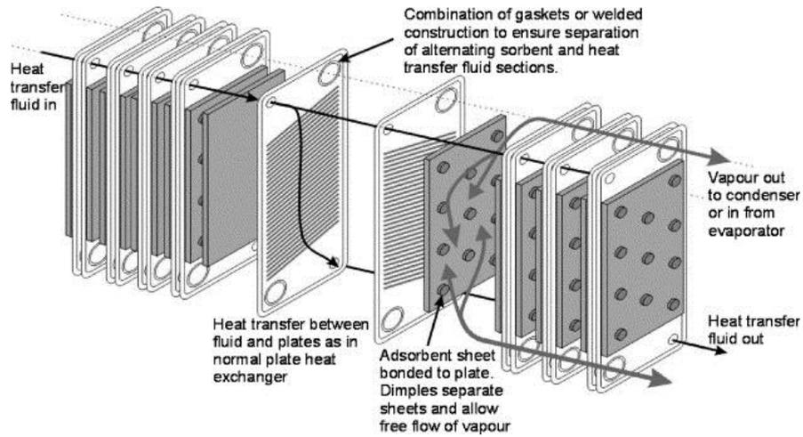
**Figure 3.24. Plate-type adsorber/desorber (Critoph and Metcalf, 2004)**
