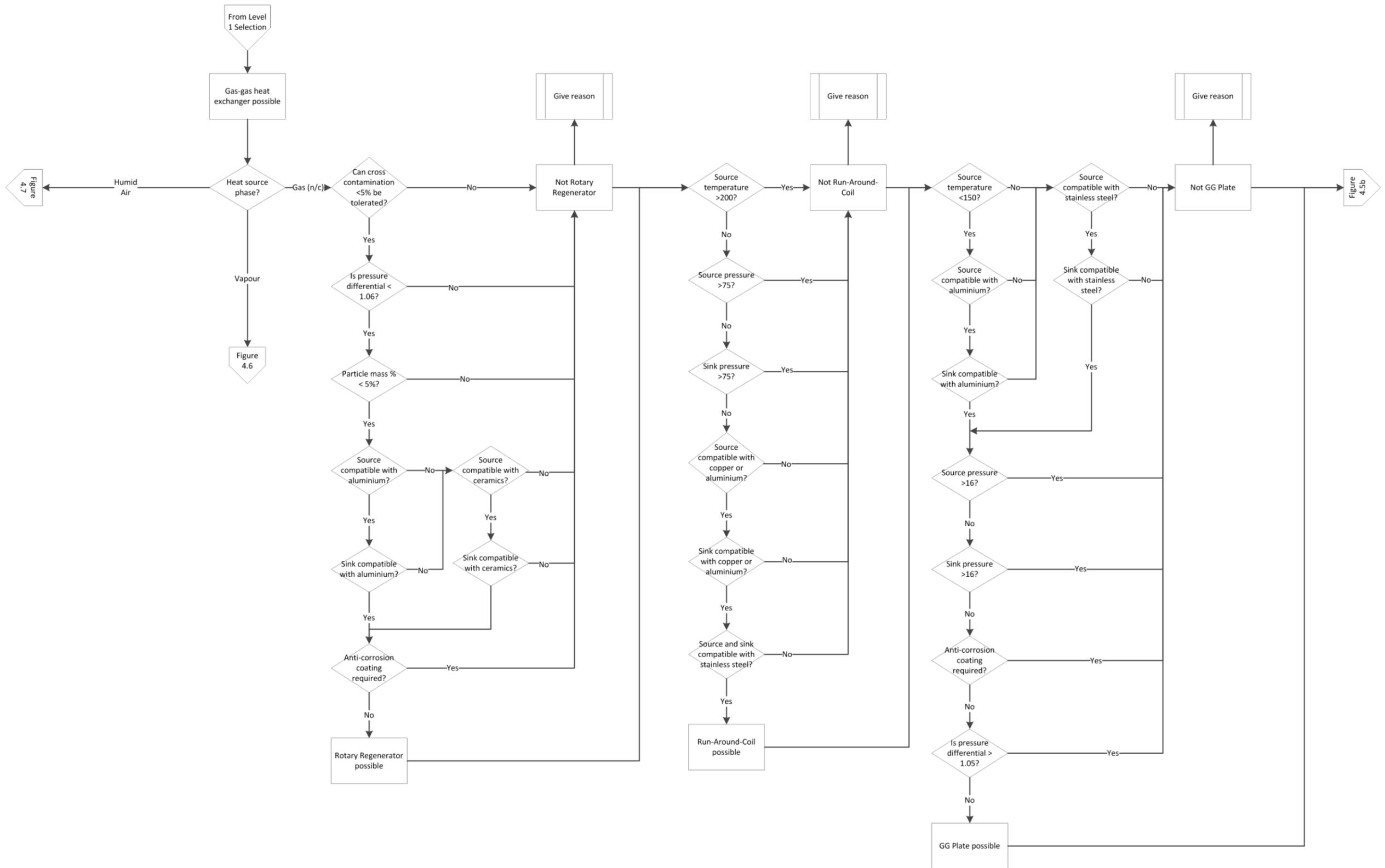
Figure 4.5. Gas-gas heat exchanger selection knowledge-base for non-condensing heat sources (part a)
