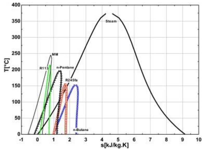
**Figure 3.19. Temperature-entropy plot for steam and several organic working fluids (Tchanche *et al*, 2011)**
