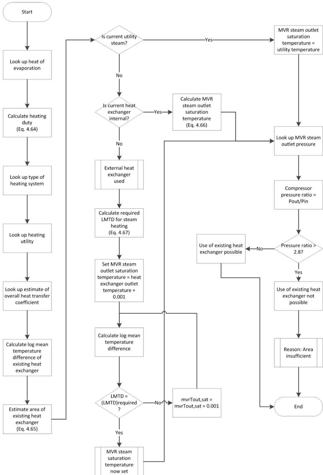
Figure 4.25. Routine to assess current heat exchanger suitability for MVR system
