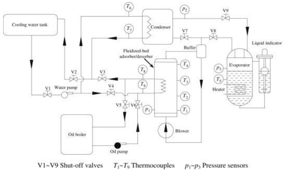
**Figure 3.23. Fluidised bed adsorption refrigeration system (Wang *et al*, 2012)**
