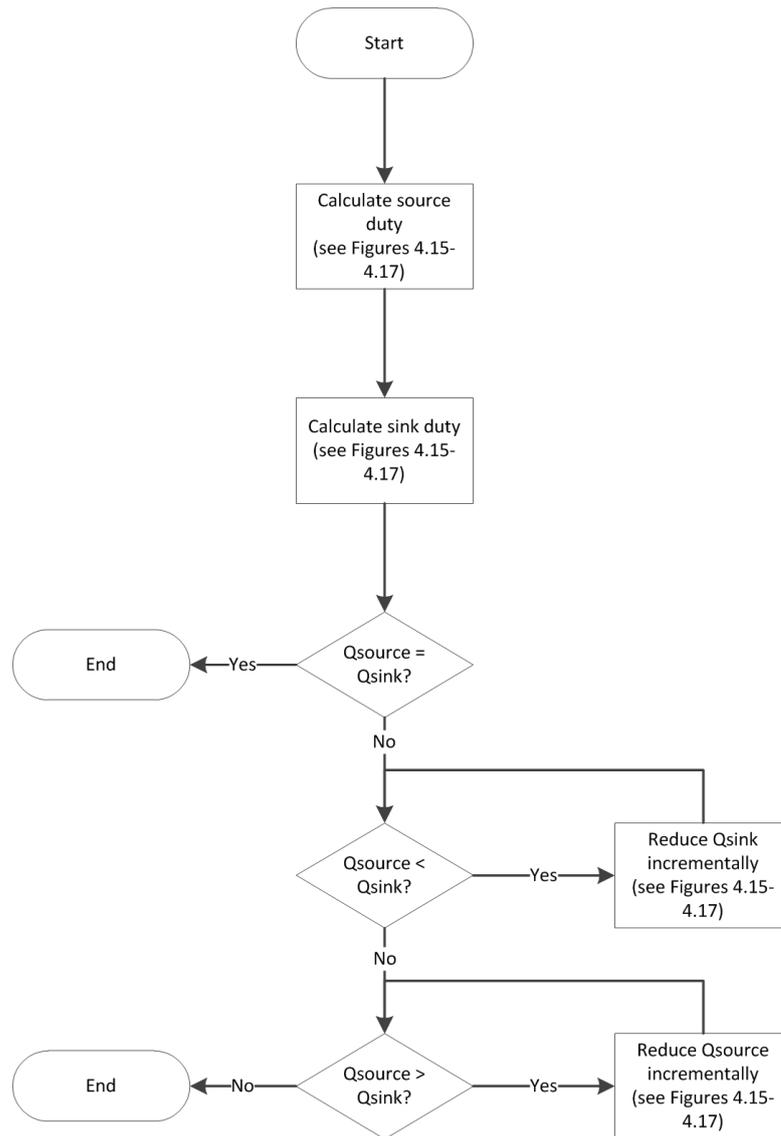
**Figure A4.1. Routine to calculate the heat balance in heat exchanger design (previously Figure 4.14)**
