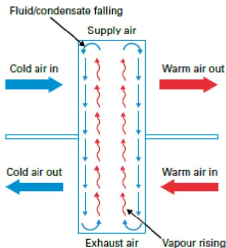
Figure 3.5. Heat pipe heat exchanger (Carbon Trust, 2012)
