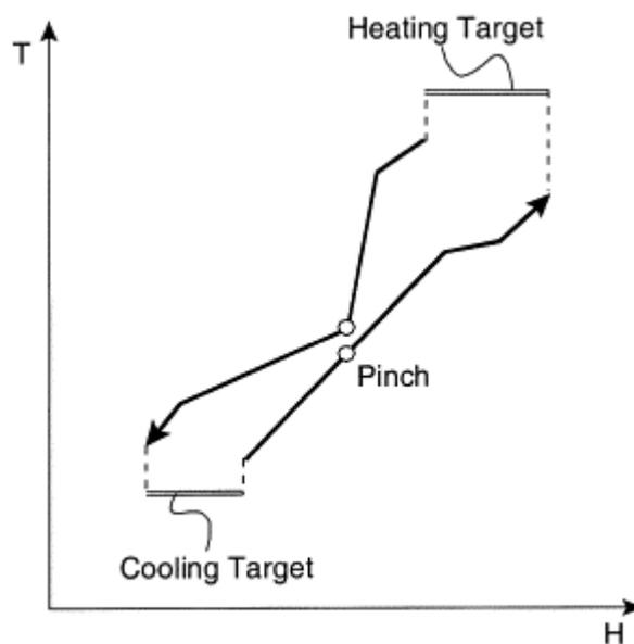
**Figure 2.1. Composite curves and pinch point (Smith, 2000)**
