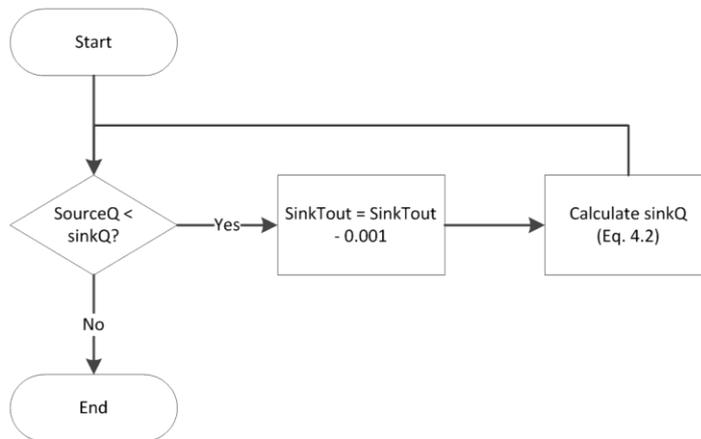
**Figure A2.2. Routing to calculate heating duties and reduce duty incrementally when no phase change occurs**
