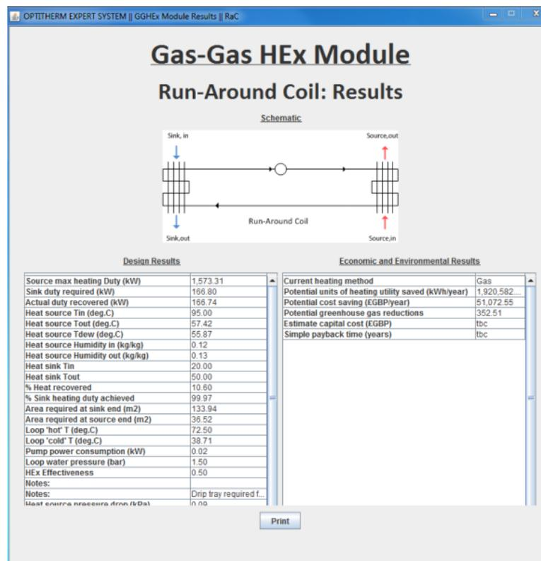
Figure A5.18. Run-around-coil heat exchanger design results for case study
