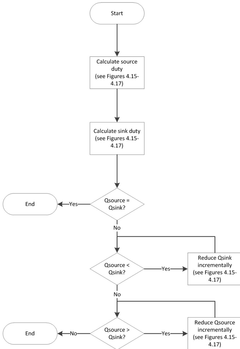
**Figure 4.14. Routine to calculate the heat balance in heat exchanger design**
