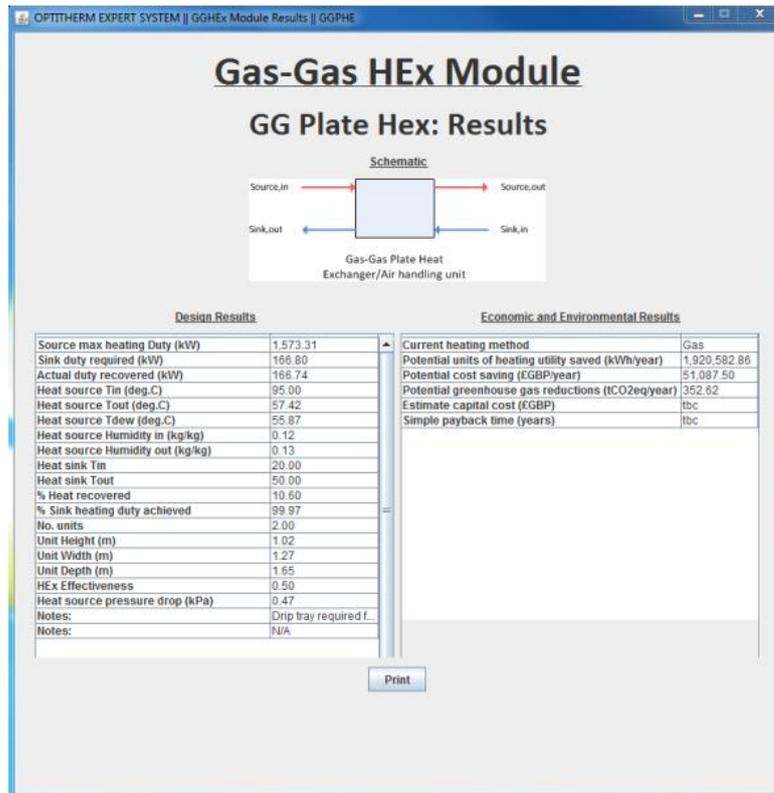
Figure A5.18. GG plate heat exchanger design results for case study
