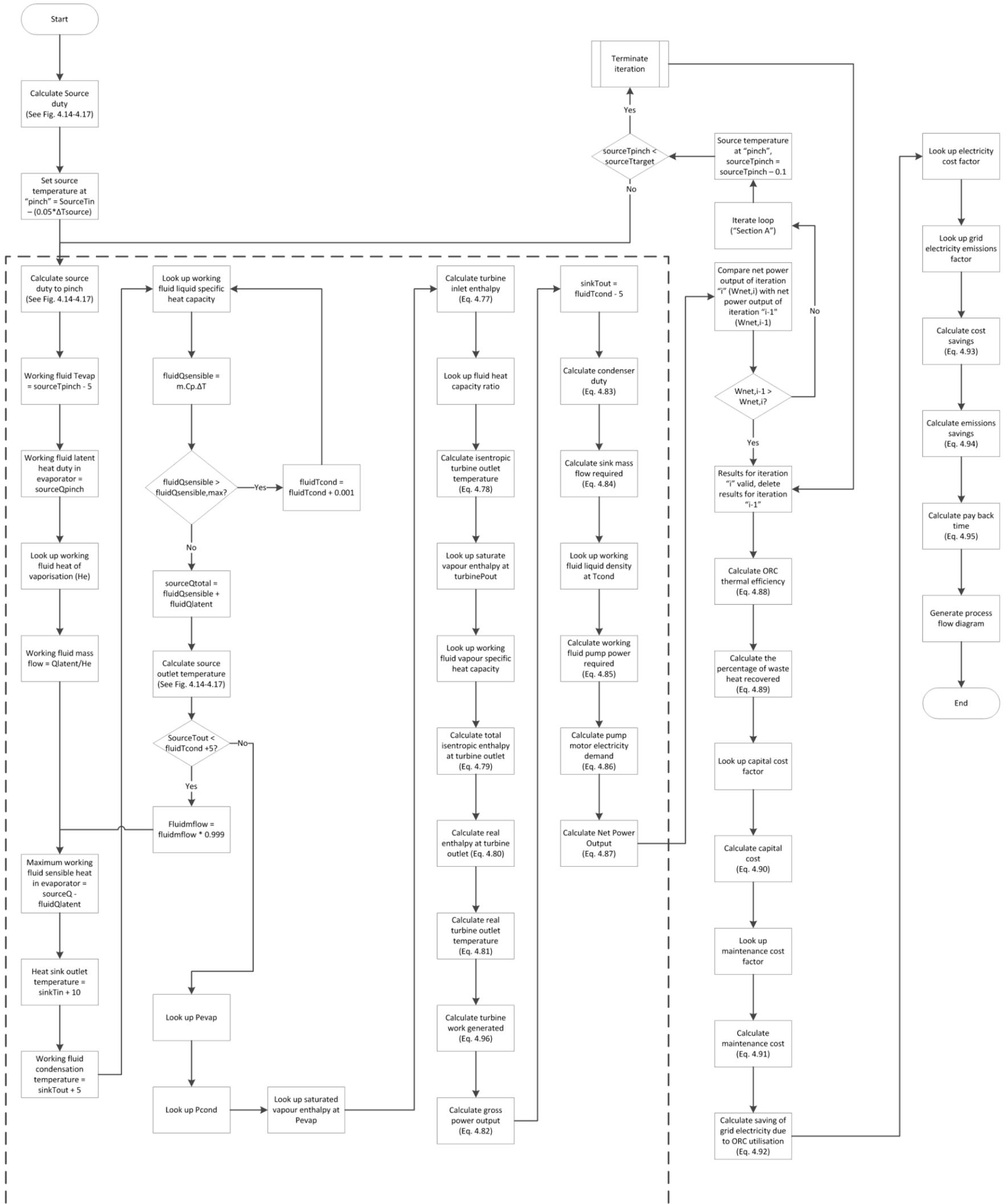
Figure 4.28. Design routine for ORC with heat sources containing sensible heat only or humid air heat sources
