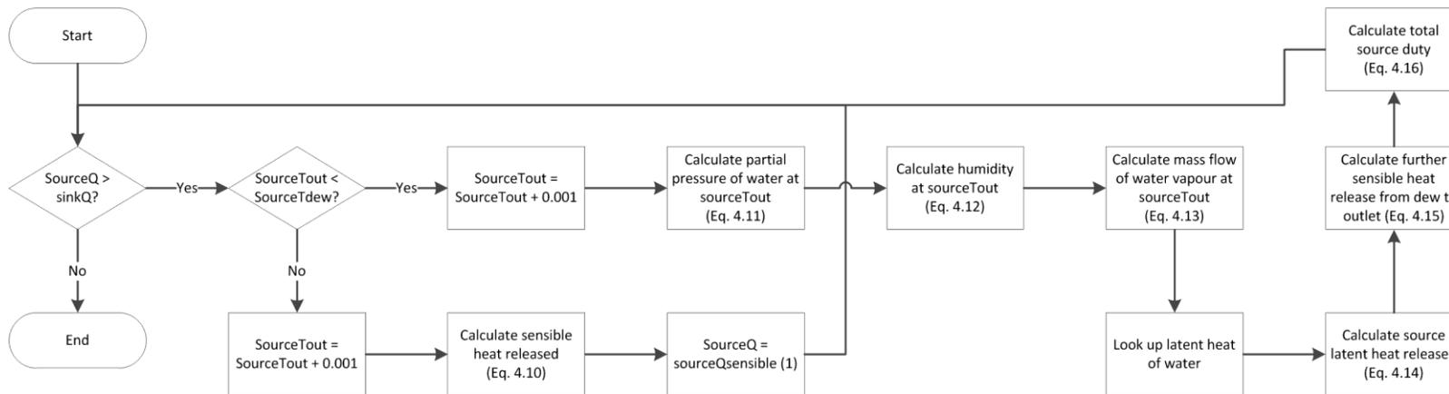
**Figure 4.17. Routine to calculate heating duty and reduce duty incrementally for a humid air heat source**
