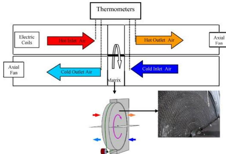
**Figure 3.2. Schematic of the rotary-regenerator (Sanaye *et al*, 2008)**
