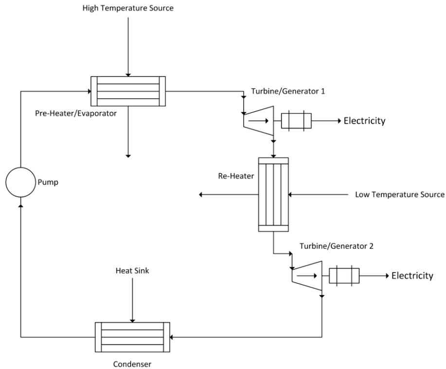
**Figure 6.3. Dual source ORC using a dual turbine re-heat cycle (adapted from Aneke *et al*, 2012)**
