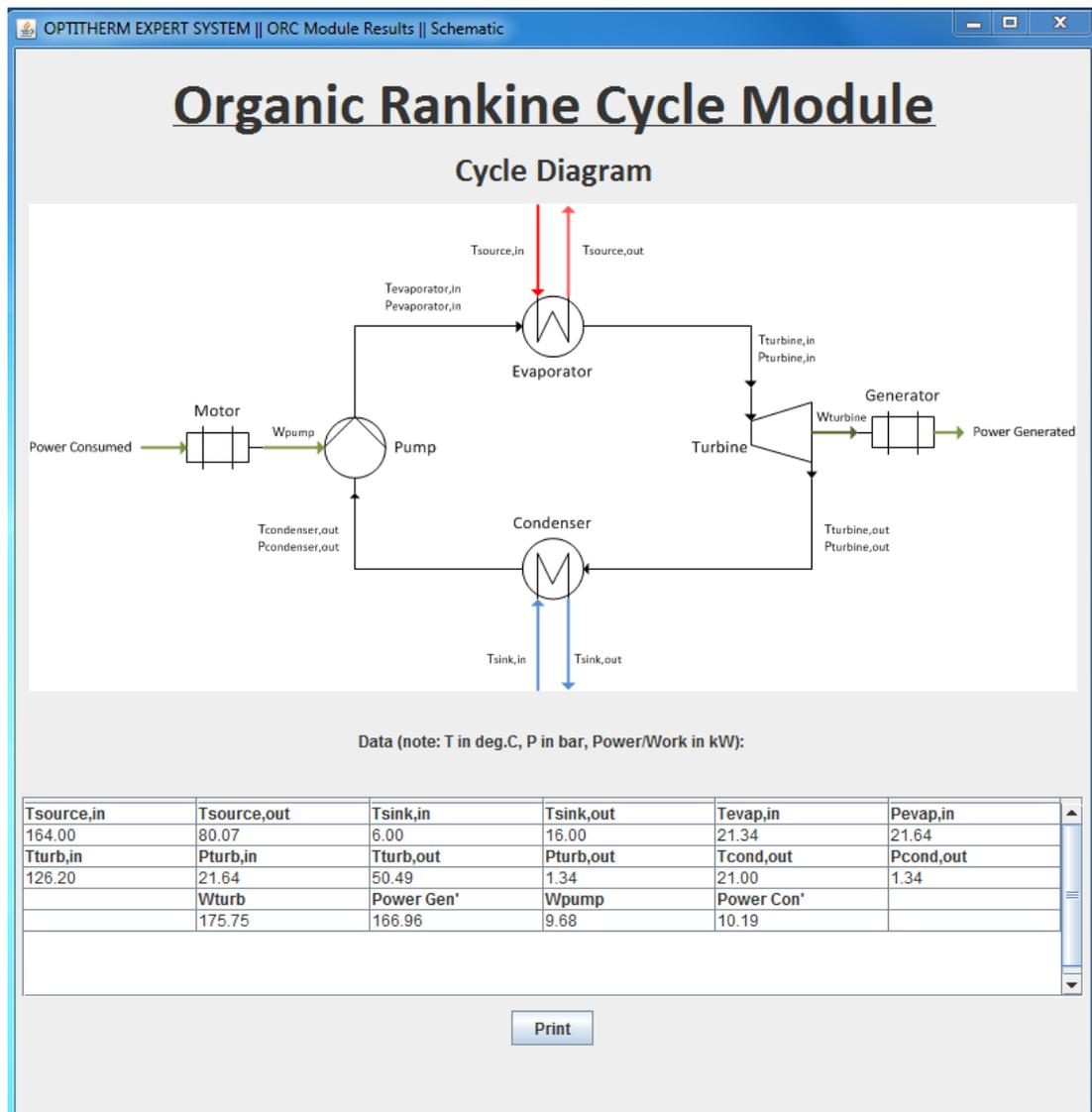
**Figure 5.5. KBS process flow diagram of results (ORC)**
