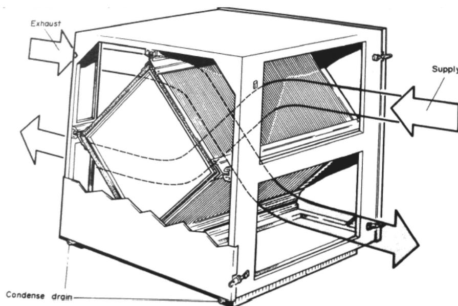
**Figure 3.1. Typical gas-gas plate heat exchanger configurations (Reay, 1979)**
