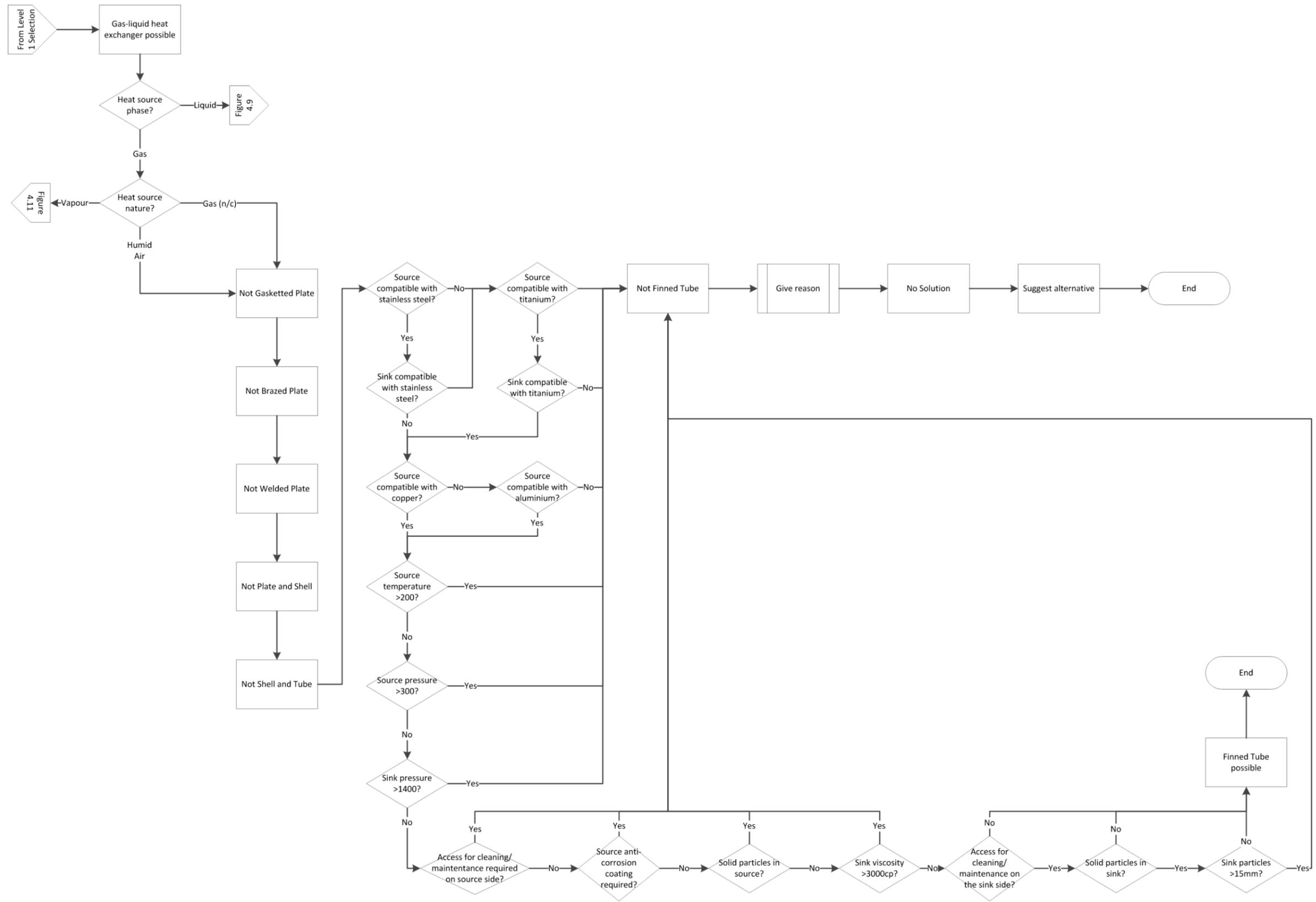
Figure 4.10. Gas-liquid heat exchanger selection knowledge-base for n/c gas and humid air heat sources
