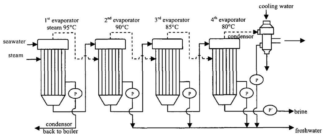
**Figure 3.26. Waste heat driven MED (Van der Bruggen and Vandecasteele, 2002)**
