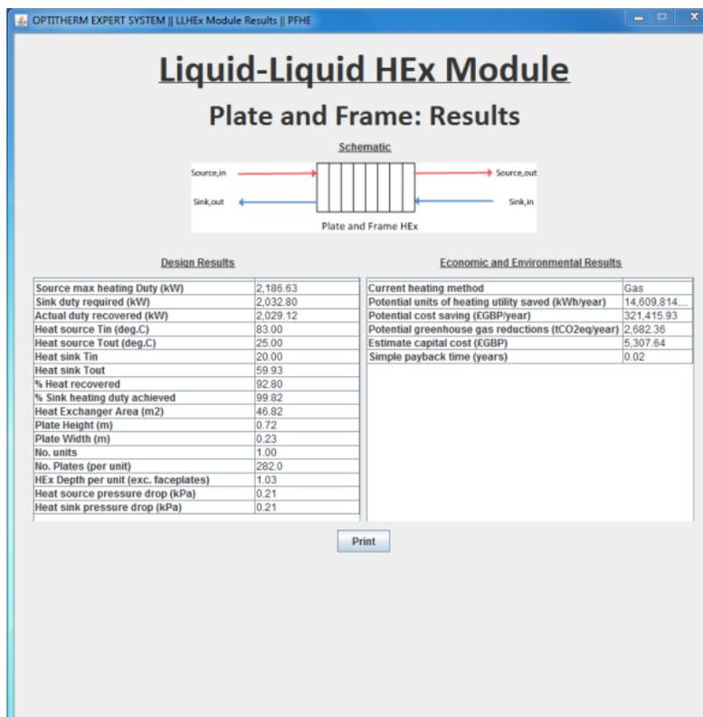
Figure A5.7. Plate and frame heat exchanger design results for case study
