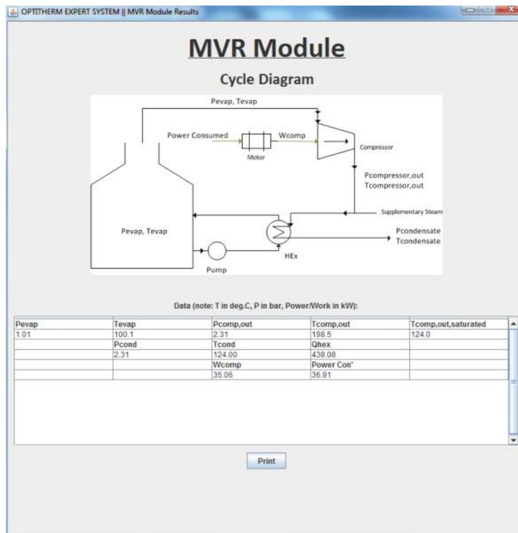
Figure A5.14. MVR (open) cycle diagram for case study
