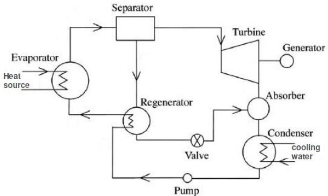
**Figure 3.21. Kalina cycle (adapted from Rotunds, 2013)**
