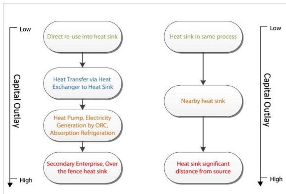
**Figure 4.4. Typical technology selection logic in waste heat recovery system design (Law *et al*, 2013)**
