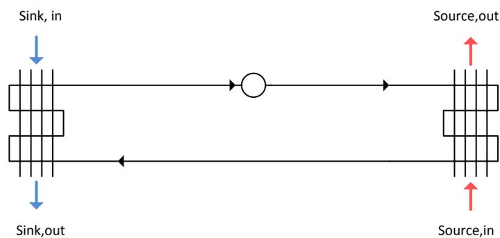
**Figure 3.4. Typical run-around-coil configuration**
