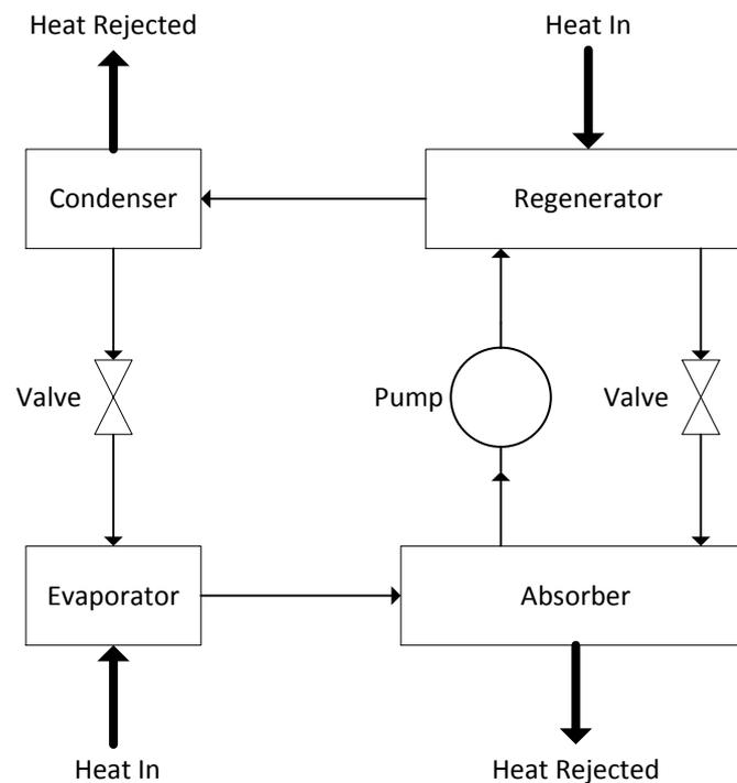
**Figure 3.22. Single-effect absorption cycle (adapted from Herold and Radermacher *et al*, 1996)**
