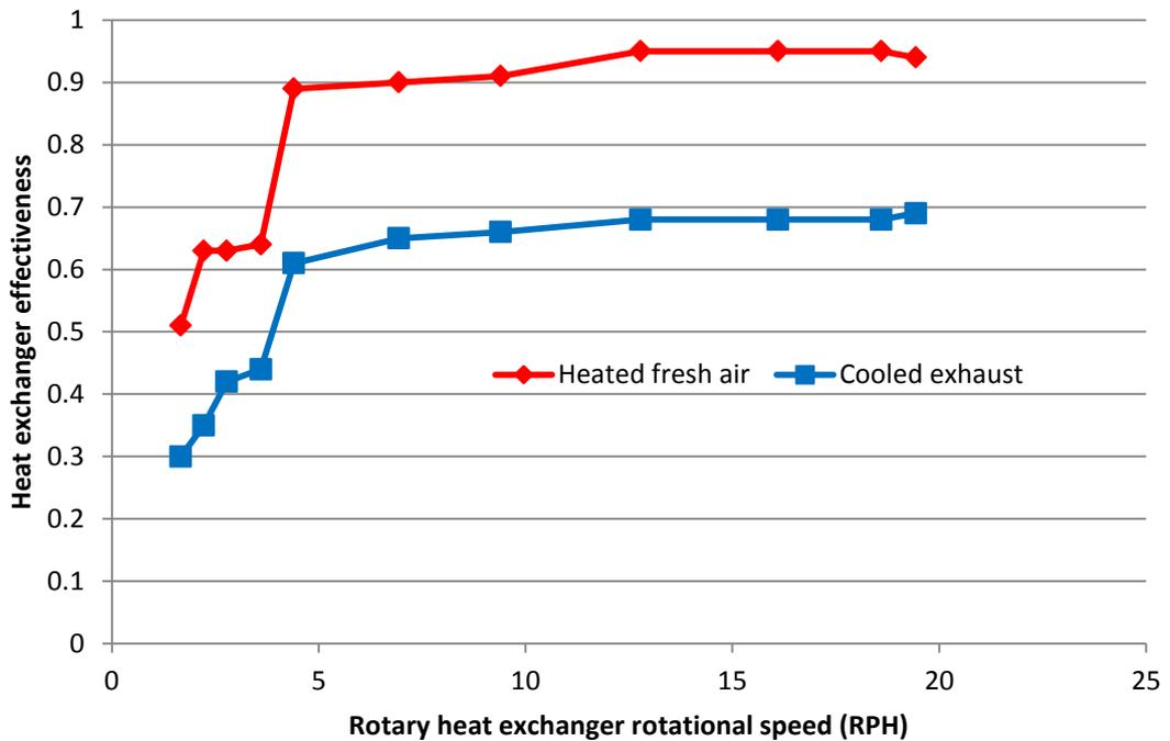
**Figure 3.3. Rotary regenerator efficiency (adapted from International Energy Agency, 1998)**
