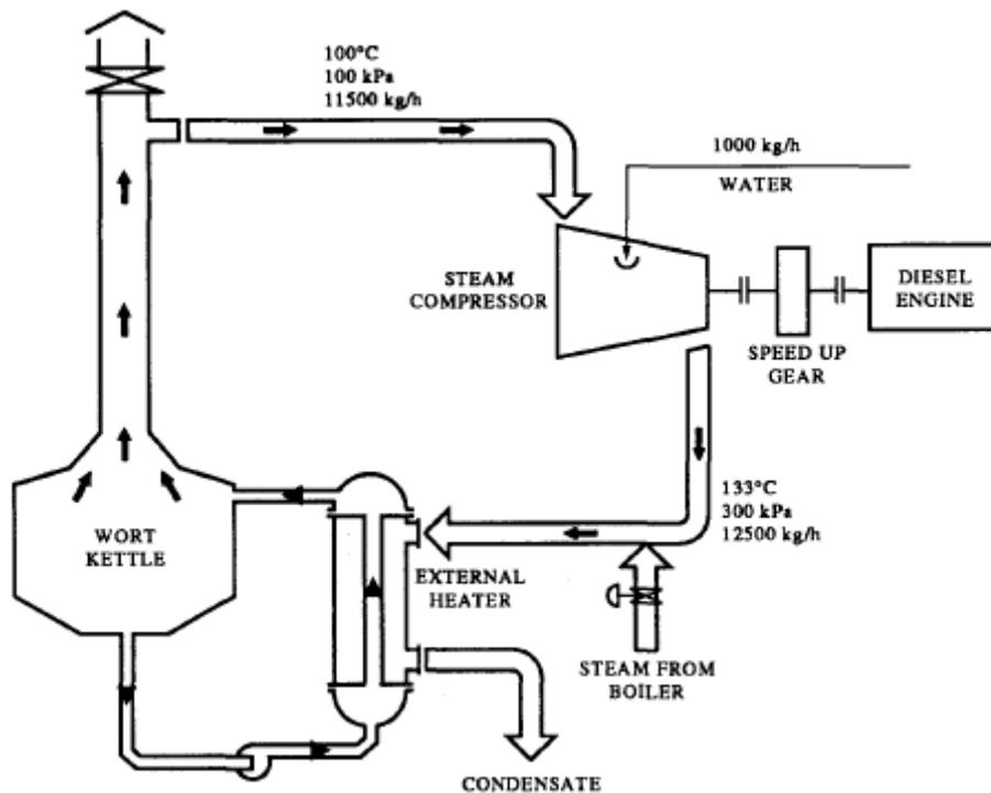
**Figure 3.16. Typical MVR installation (Lazzarin, 1993)**
