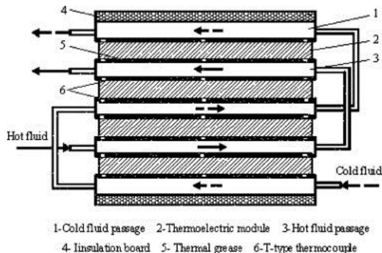
**Figure 3.18. Thermoelectric device (Nie *et al*, 2011)**
