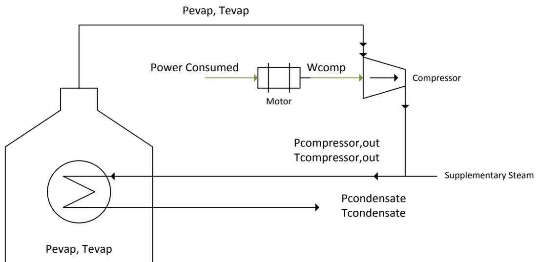
**Figure 4.22. Standard MVR configuration with internal heating coils**
