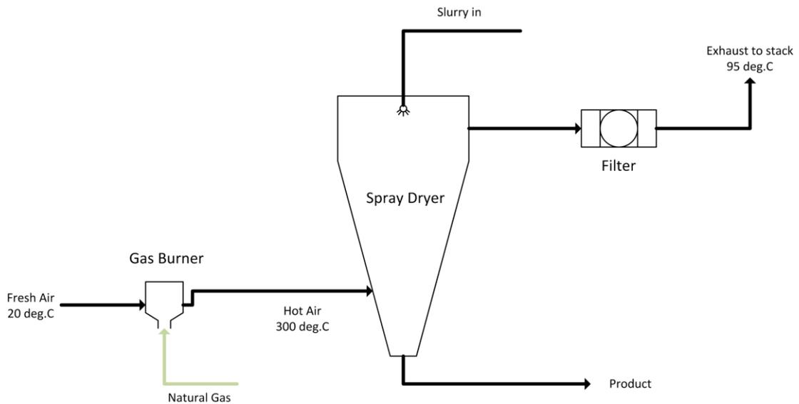
**Figure 6.7. Spray dryer process from case study 5**
