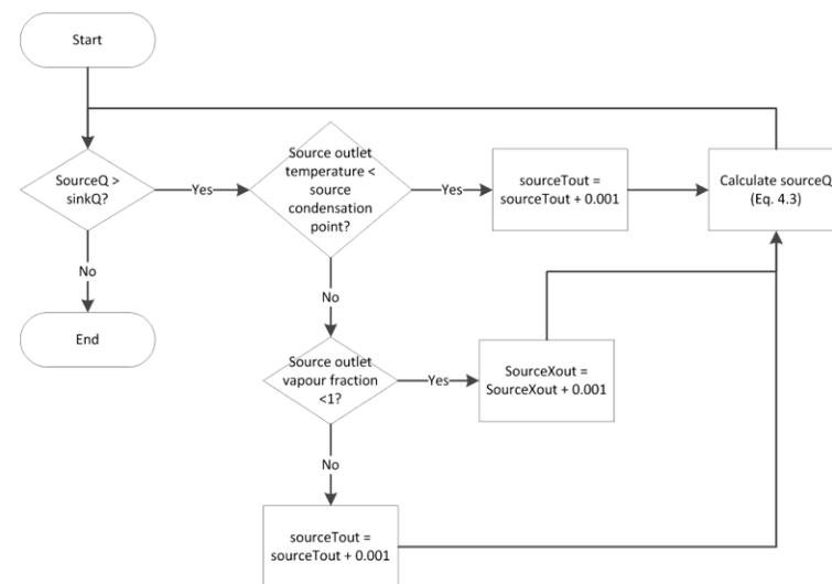
**Figure 4.16. Routine to calculate heating duties and reduce duty incrementally when boiling or condensation occurs**
