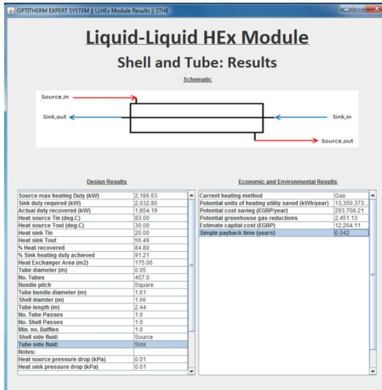
Figure A5.6. Shell and tube heat exchanger design results for case study
