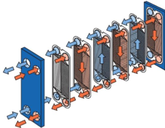
**Figure 3.7. Plate heat exchanger flow configuration (Alfa Laval, 2013)**
