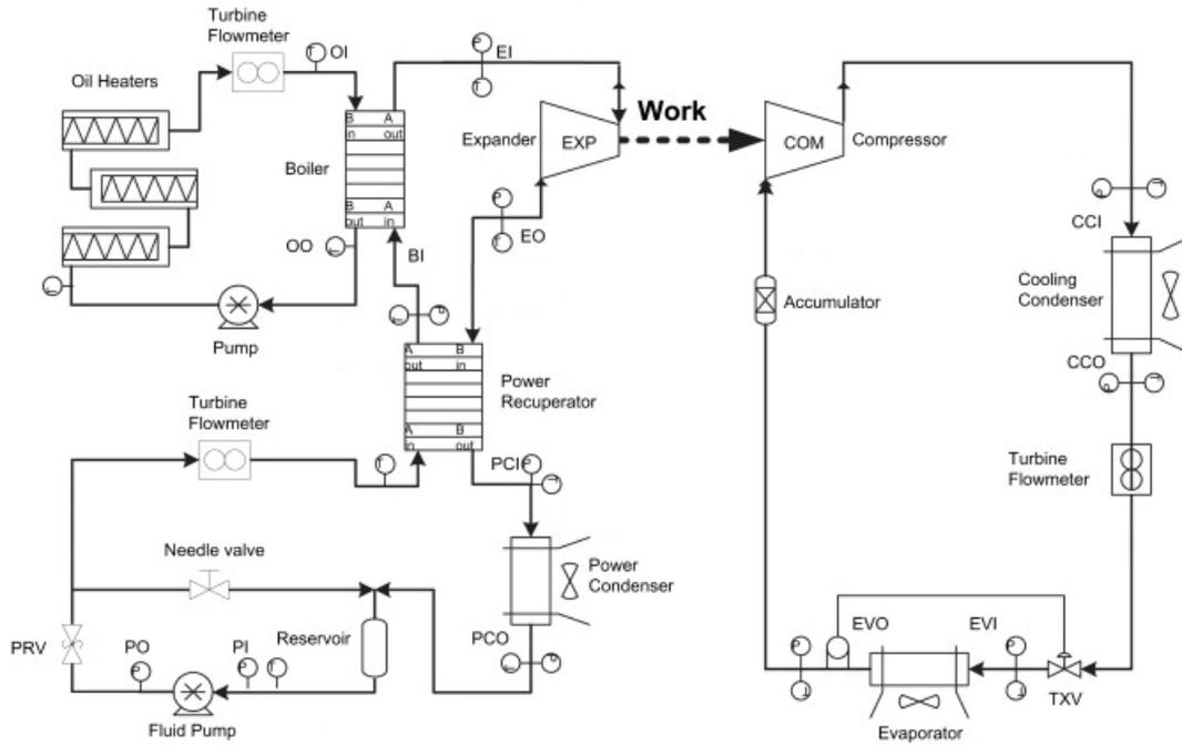
**Figure 3.25. Schematic of ORC-VC refrigeration system (Wang *et al*, 2011)**
