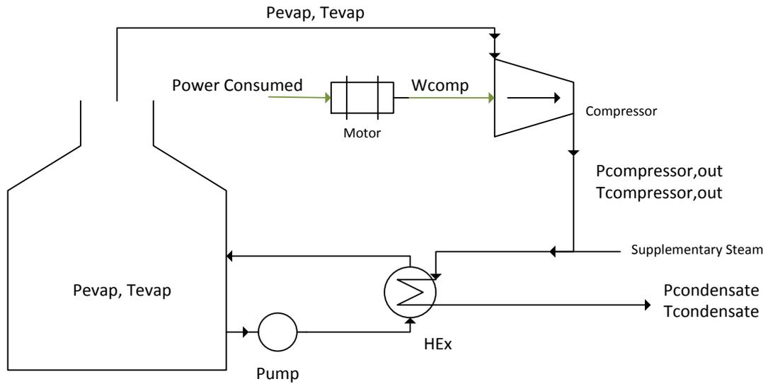
**Figure 4.23. Standard MVR configuration with an external recirculation heat exchanger**
