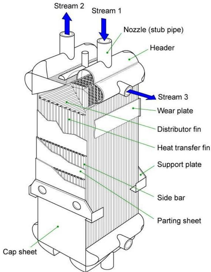
**Figure 3.13. Plate-fin heat exchanger configuration (Best Practice Programme, 2000)**
