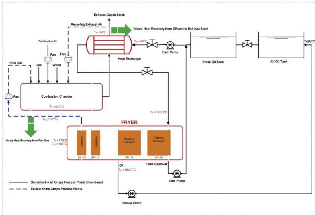
**Figure 6.1. Process flow diagram of “fryer” from case study 1(Aneke *et al*, 2012)**
