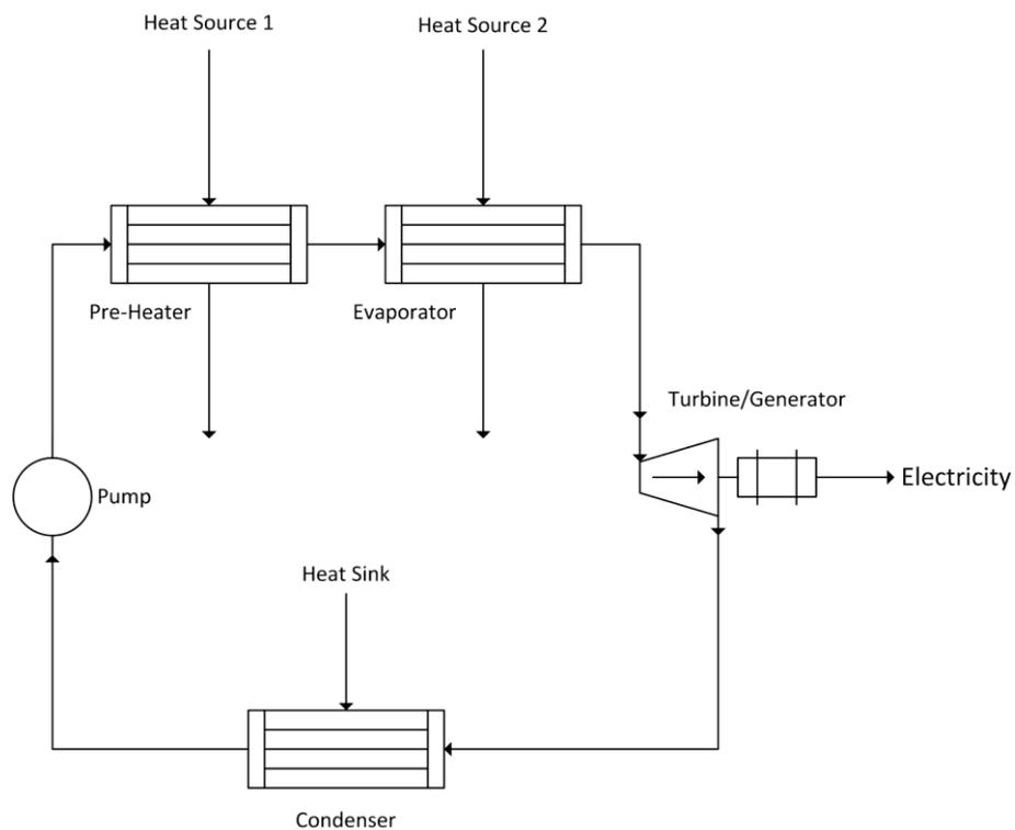
**Figure 6.2. Dual source ORC using two heat exchangers in parallel (adapted from Aneke et al, 2012)**
