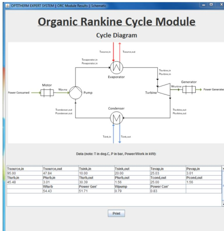
Figure A5.20. ORC cycle diagram results for case study
