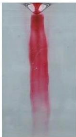
Figure 2-31: Developing cylindrical dye curtain below the vortex using a magnetic bar stirrer (Halász et al. , 2007)
