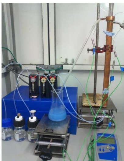
Figure 4-66: Pale blue precipitation observed from the outflow of the solvent-free reaction of benzaldehyde and n -butylamine conducted using the thermosyphon mesoscale-OBR
