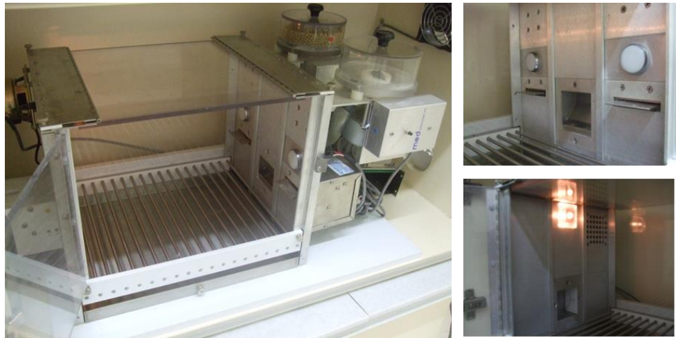
Figure 2-2 Photographs of the operant chamber. The photographs show the operant box (left), the levers and magazine (top right) and the speaker and house light (bottom right).
