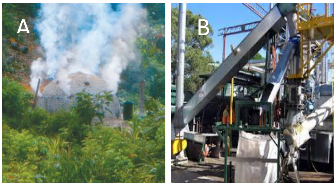
Figure 2.2: Manual oven (A) and Industrial pyrolysis unit (B) for Biochar production
