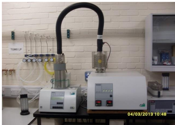
Figure 3.3: Coupled thermogravimetric, differential scanning calorimetric and quadrupole mass spectrometry System
