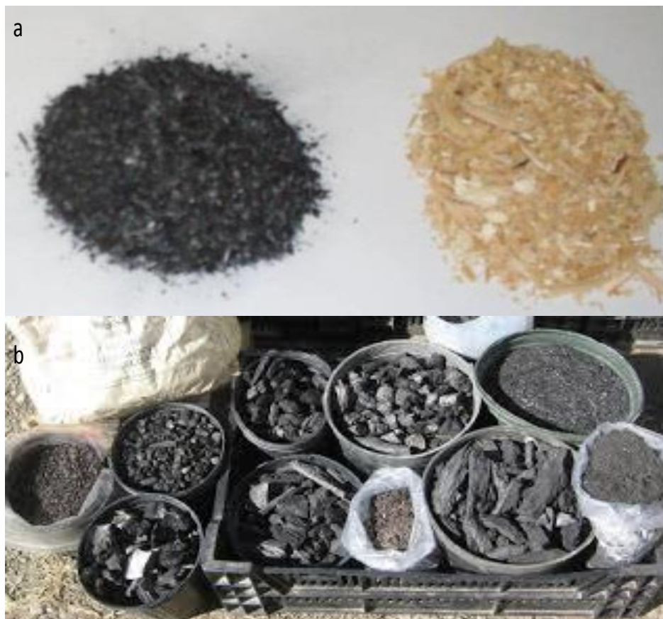
Figure 1.1 (a) Sitka spruce wood chips (right) and its biochar (left), (b) biochar products from various feedstock sources such as rice husk, corn cobs, wheat straw, saw dust and chicken manure.
