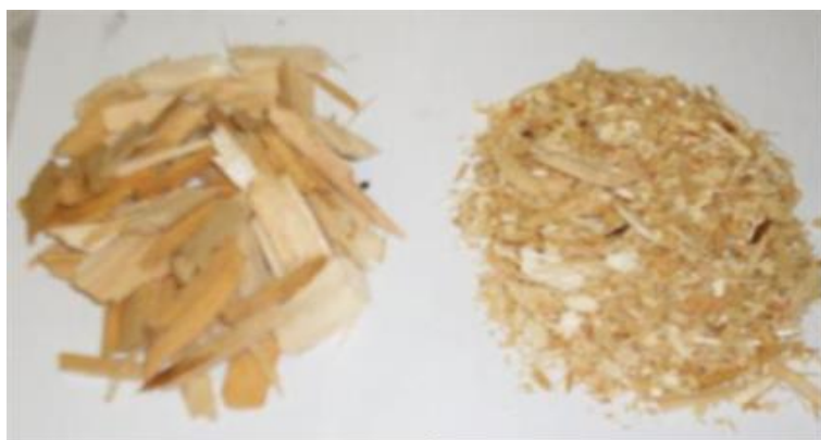
Figure 3.1: Sitka spruce wood chips and saw dust processed to produce the biochars studied.
