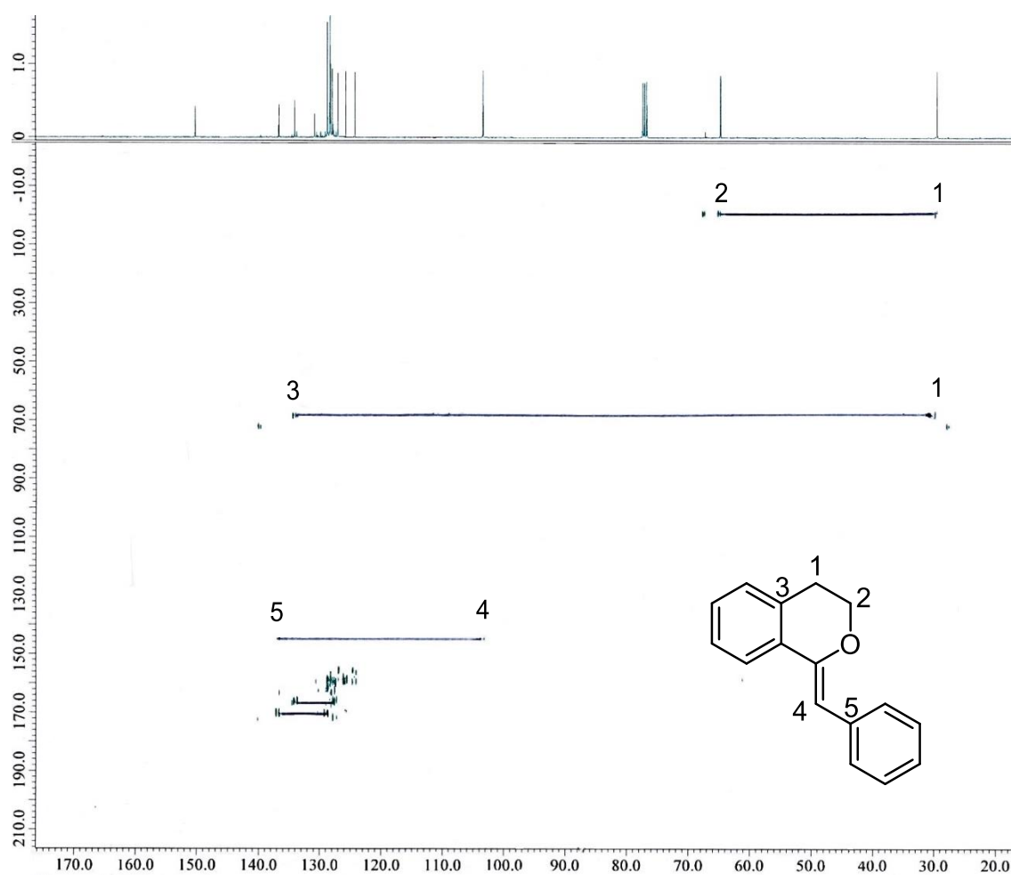
Figure 39. The INADEQUATE experiment used to determine the structure of (Z)-1-benzylideneisochromane 74 . This experiment was performed using the JEOL ECS 400 NMR instrument.
