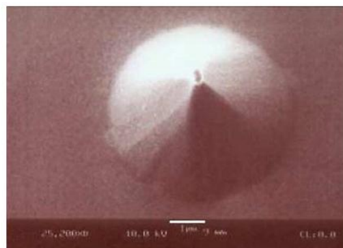
Figure 1-6: The fine tunneling tip of tunneling MEMS microaccelerometer. The scale bar being 1 \mu\text{m} . Taken from (Dong, Jia et al. 2005).
