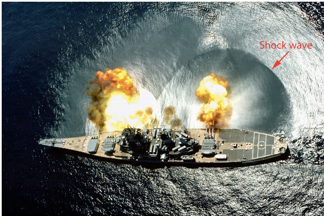
Figure 5-1. Shock wave depicted from the main weapon of a warship. The shock wave can be seen with the blast wind and finally the flame from the explosion.
