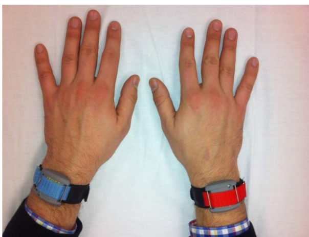
Figure 23: Axivity AX3 devices mounted in Velcro straps (colour coded to indicate the hand on which they were to be worn; red: right, blue: left)
