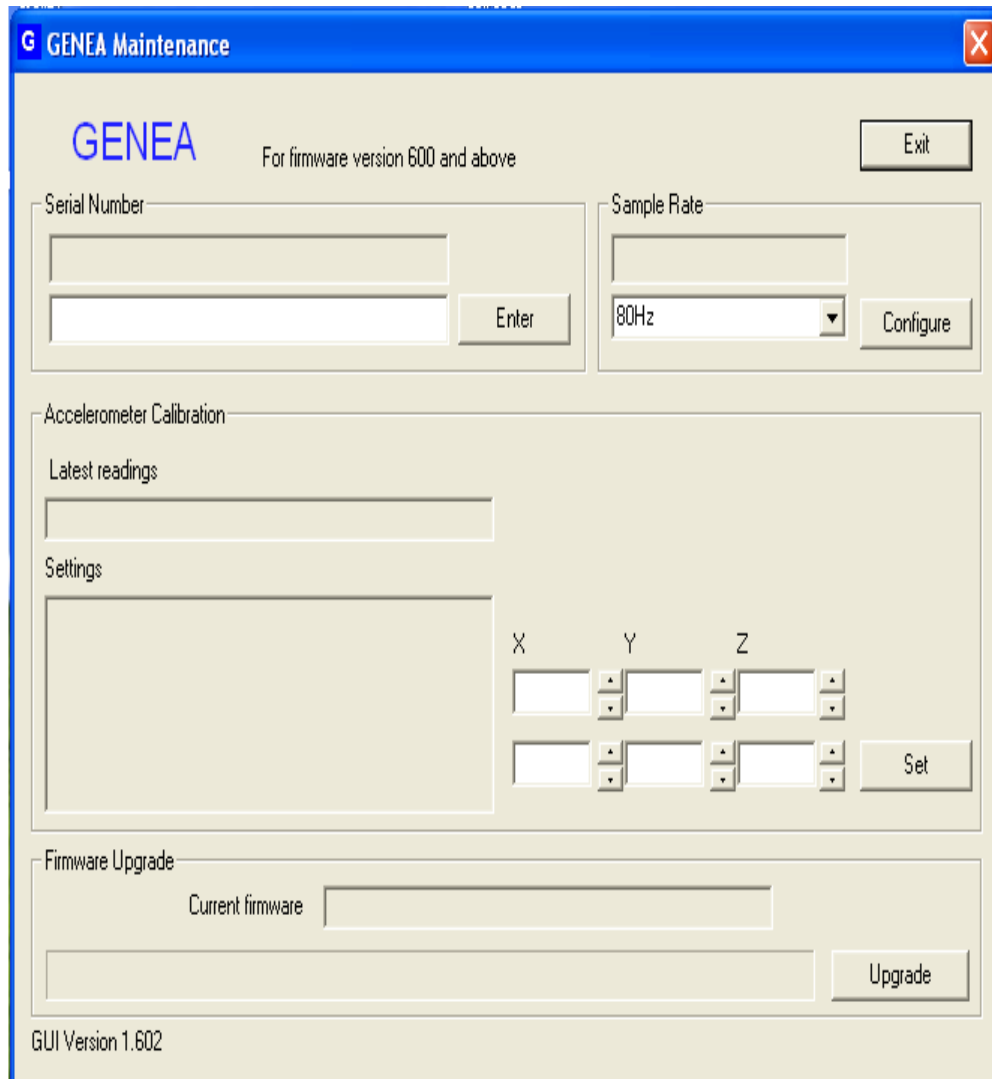
Figure 3.4 : Screen shot of accompanying software which allows configuring sampling frequency and setting an offset for the accelerometer.
