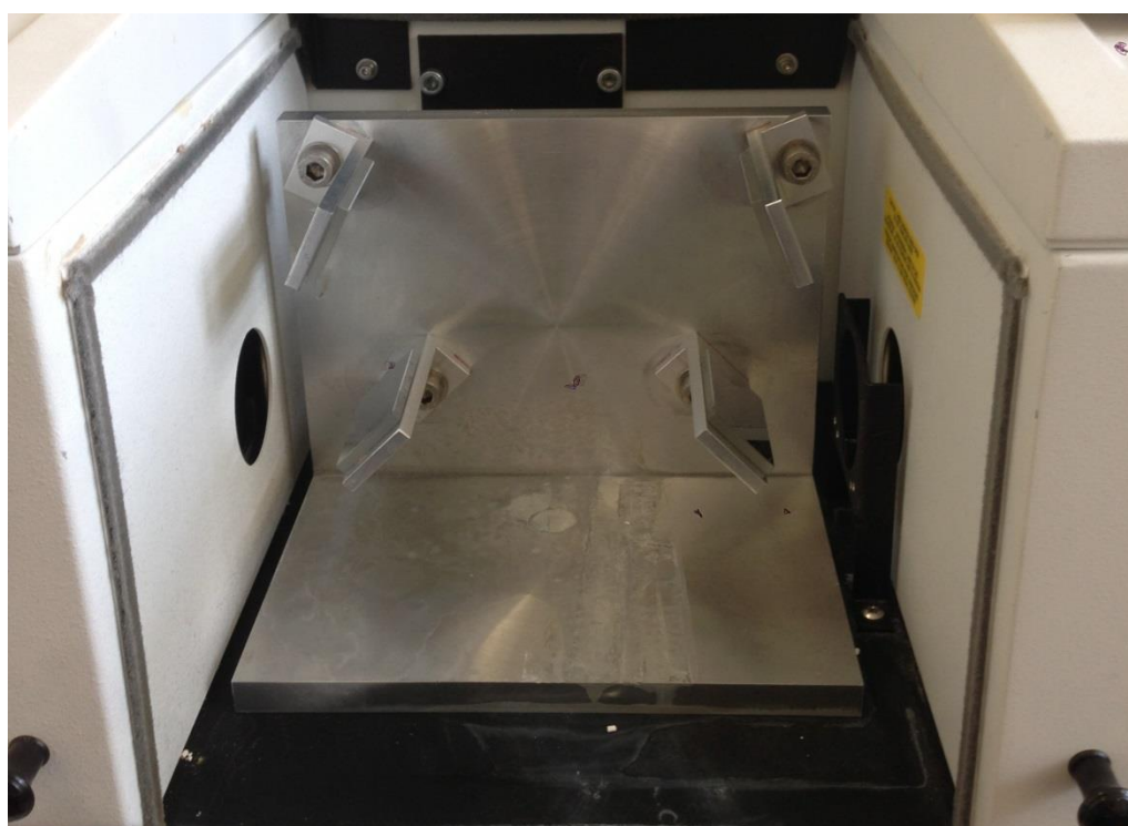
Figure 2.6. (a) Schematic and (b) photograph of the mirror configuration within the FTIR sample compartment, thus allowing for reflectance of the IR beam at the Pt working electrode.
