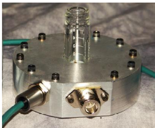
Figure 3: Typical laboratory microwave reaction cavity and infrared thermometer containing a 5 mL reaction vial (Resonance Instruments Inc., 2011)
