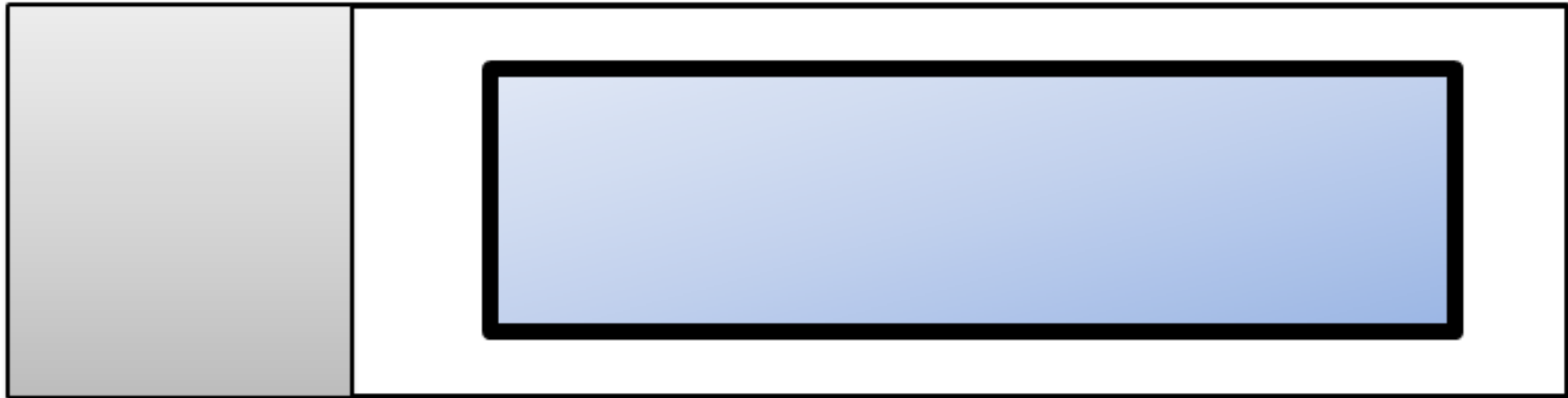
Figure 3.1 Illustrative example of a membrane slide with the membrane highlighted in faded blue and the black exterior of the membrane representing the hydrophobic layer used to isolate cells for single cell analyses
