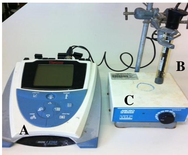
Figure 3.2 The ion selective electrode measures fluoride release in millivolts; a) Ion meter, b) Ion selective electrode, c) Magnetic stirrer.
