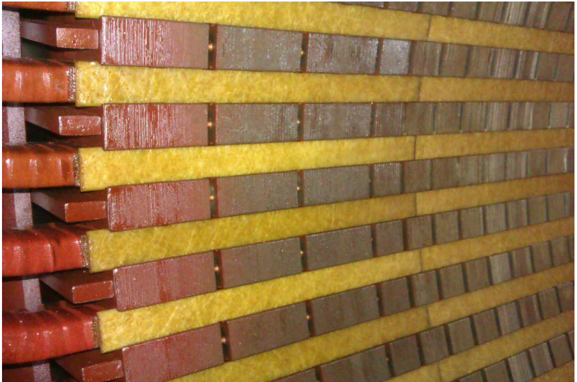
Figure 26 – Photograph of Machine Radial Ventilation Ducts
