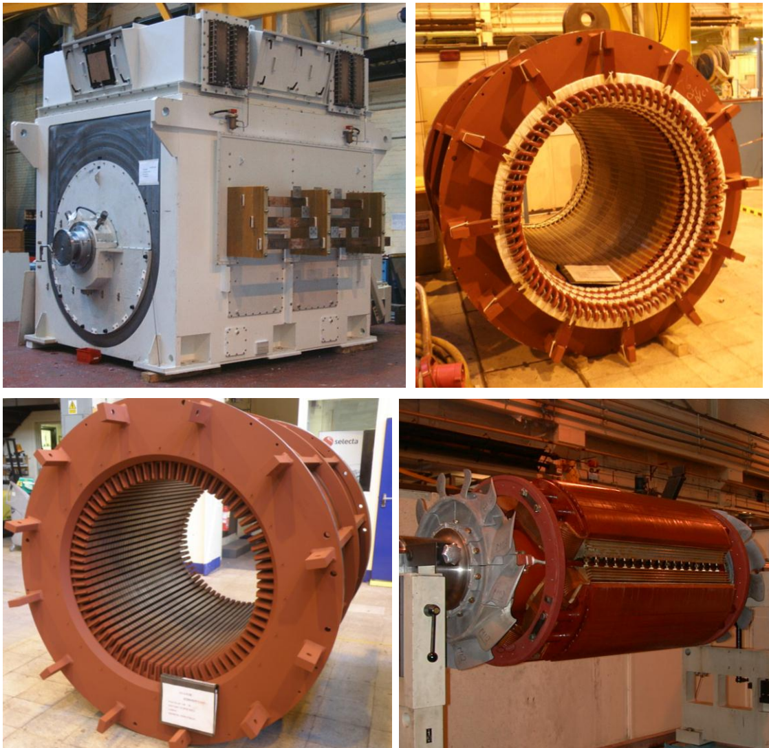
Figure 129- Several multi-megawatt generators at various stages of construction
