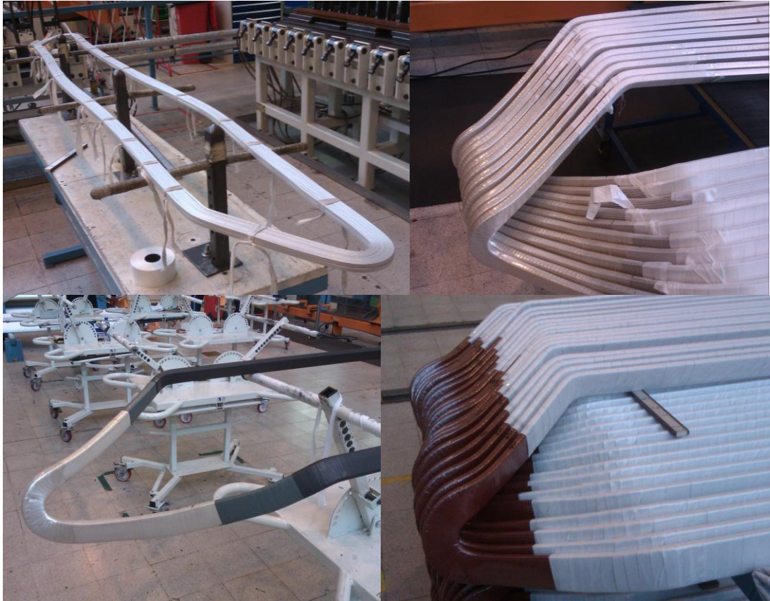
Figure 9 - Coils at various stage of construction:
