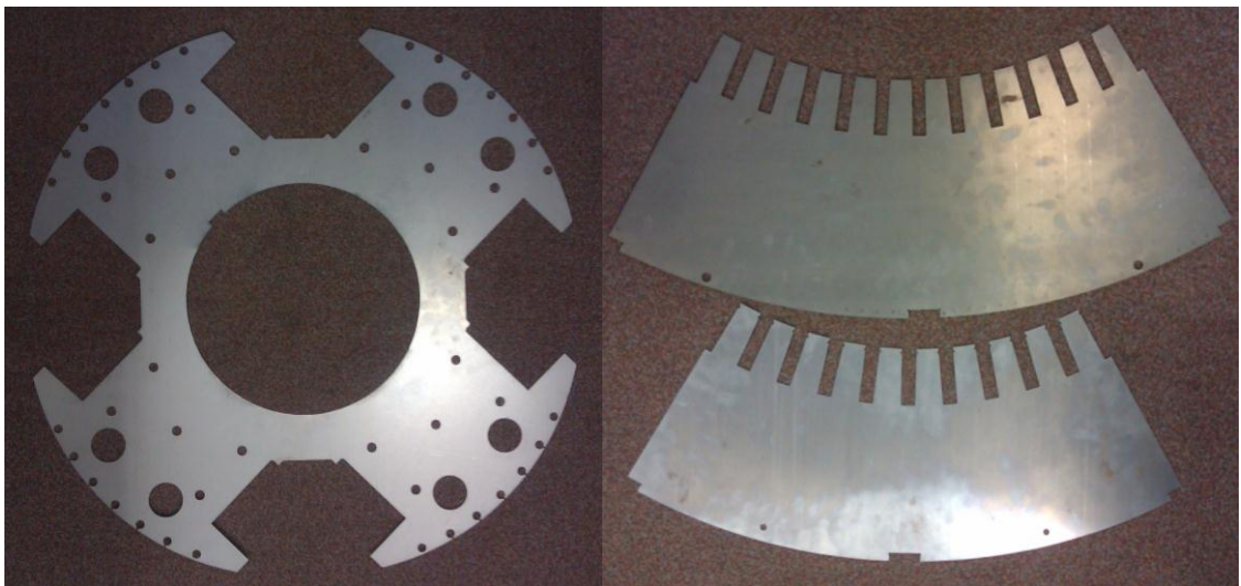
Figure 7 - Photographs of wound field synchronous generator laminations: Left - 4 pole rotor lamination from the A183 range (1.15m rotor diameter). Right - segmental stator laminations from 2 different generators, (outside diameter 1.6 m and 1.83m)
