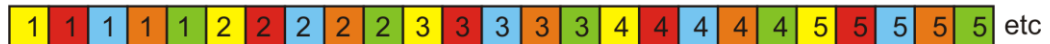
Figure 103 - Diagram showing the order that data must be arranged in a five steps per slot system.
