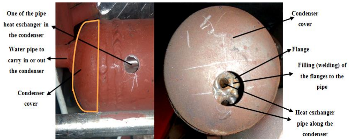
Figure 3-15: The condenser's heat exchanger
