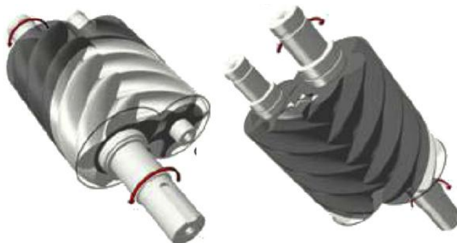
Figure 2-19: Screw set operation principles
